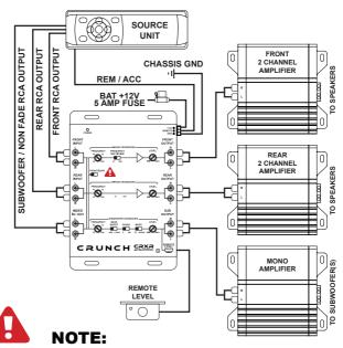
For 5 Channel source unit operation, be sure the "REAR INPUT" switch is in the **REAR**
