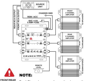
For 4 Channel source unit operation, be sure the "REAR INPUT" switch is in the **REAR** position.
