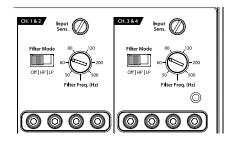
To properly set the amplifier for maximum clean output, please refer to Appendix A (page 14) in this manual. After using this procedure, you can then adjust any or all "**Input Sens.**" levels downward if this is required to achieve the desired system balance.
