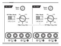
1) "Filter Mode" Controls: The M700/5 employs 12dB per octave filters for each pair of main channels (one high-pass filter for channels 1&2 and another high-pass / bandpass filter for channels 3&4. The Subwoofer Channel provides a low-pass filter with the option of 12dB or 24dB / octave slopes. Each of these filters can be controlled or defeated completely by way of the three-position "Filter Mode" switches in each Channel Section:
