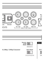
If you wish to send six discrete channels into the M700/5, simply use all six inputs and set the "Input Mode" switch in the "6 Ch." position. The amplifier will automatically combine the Sub Ch. input signals to mono.
