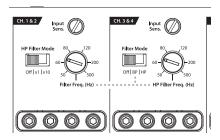
To properly set the amplifier for maximum clean output, please refer to Appendix A (page 14) in this manual. After using this procedure, you can then adjust any or all "Input Sens." levels downward if this is required to achieve the desired system balance.
