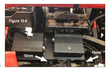
Connect the power and speaker wiring to the harness as labeled. Do not zip-tie anything at this point as the dual
