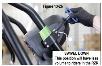
Once the general mounting position is chosen, do not fully tighten the pods as you may want to do final adjustments for your ear height after the seat is in position and the system is playing music.
