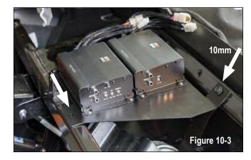
You will tighten the 16mm nuts and washers next to the steering column once reassembly of the vehicle begins. This allows easy removal of the amplifier plate for troubleshooting (if necessary).
