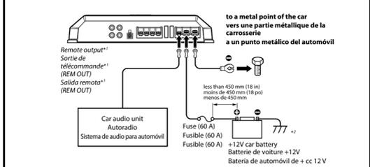
\*1 If you have the factory original or some other car audio unit without a remote output for the amplifier, connect the remote input terminal (REMOTE) to the accessory power supply.
