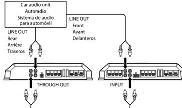
When you connect amplifiers using the THROUGH OUT pin jacks, it allows you to connect up to a maximum of three. Otherwise the necessary output levels cannot be obtained, and your car audio unit may be damaged.
