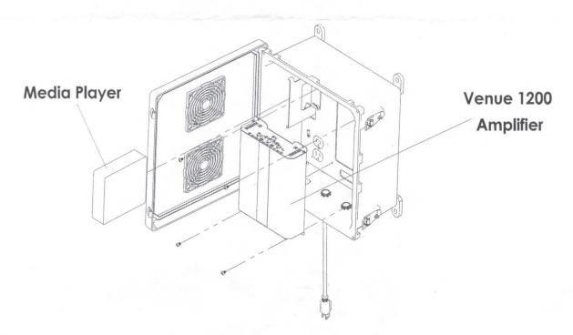
**Step 3)** Refer to amplifier manual and complete wiring of all components. Once all components installed and wired, the outdoor enclosure is ready to be plugged in for operation.
