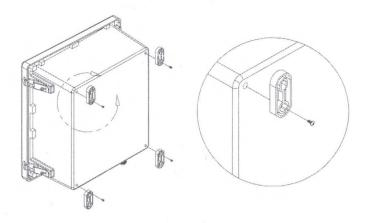
**Step 2)** Install Venue 1200 Series Outdoor Amplifier using included hardware. Slide media player into side bracket (media player not included), snug media player in place and tighten down included hardware.
