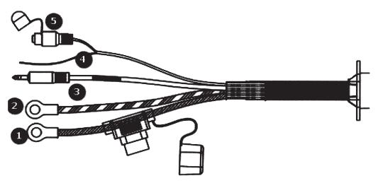
**IF INSTALLING ON A GAS OR DIESEL VEHICLE** – wire the Negative (Black) wire (2) on the subwoofer harness to the Negative (-) battery terminal and the **Positive (Red) wire (1)** on the subwoofer harness to the Positive (+) battery terminal.
