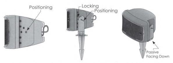
\*If using optional Ground Spike, securely mount the bracket to ground spike, place spike in desired landscape location and follow speaker mounting instructions above.
