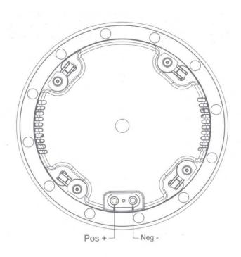
**Step 3** - Remove magnetically retained grille. Install speaker into mounting location and tighten baffle screws to engage mounting brackets. Once fully tightened, the brackets will clamp to the mounting surface securing the speaker in place.
