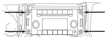
2 Release 2 clips on the top of the bottom panel. This will expose two 7mm screws. Remove those.
