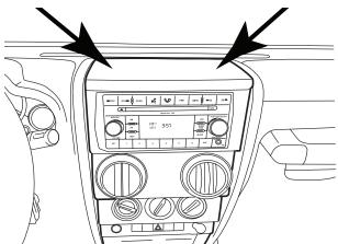
3 Release 2 clips on the top of the bottom panel. This will expose two 7mm screws. Remove using a 7mm socket with ratchet & extension.
