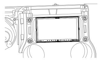
2 Attach the side brackets using the provided 8mm round head screws.
