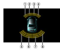
Indicator colors when an obstacle is detected. Red: close distance Orange: medium distance Yellow: long distance
