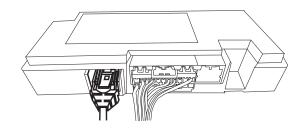
NOTE: Since the factory Uconnect® system is not going to be used you can unplug the 24 pin connector shown in step 2. If Uconnect® module is not disconnected the Uconnect® system will stay paired with previously paired phones. The user's phone may connect to both Bluetooth devices simultaneously resulting in unpredictable and potentially distracting behavior.
