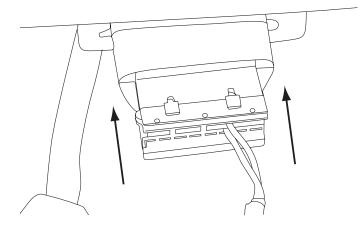
3 Mount the microphone as illustrated and run the cable to the radio cavity. You will need to use a T20 Torx to remove the visor. For optimal performance it should be mounted by the rear-view mirror as illustrated.
