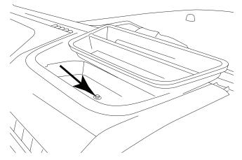
3 Remove the window switch pod using a panel removing tool and extract (1) 7mm screw.
