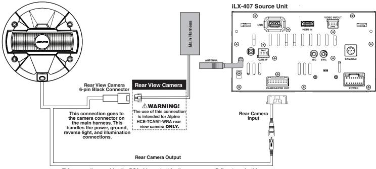
This connection provides the RCA video output for the rear camera. Failure to make this connection will result in no picture being sent to the iLX-407.
