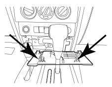
5 Extract (4) 7 mm screws and remove the factory radio.
