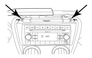
4 Use panel removal tool to remove dash panel by releasing 6 clips (3 per side)
