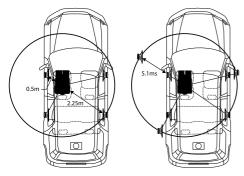
The sound is not balanced because the distance between the listening position and the various speakers is different. The difference in distance between the front left speaker and the rear right speaker is 1.75 m (68-7/8"). Here we calculate the time correction value for the front left speaker in the diagram on the above.
