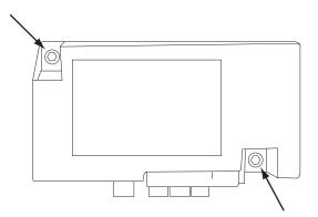
3 Secure the Uconnect® module to the original location using the 7mm bolts.
