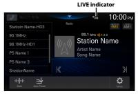
In live broadcast, such as sportscasts, etc., a time lag occurs between digital sound and analog sound. Therefore, when live broadcasts are received, a time lag between the real broadcast may occur and the unit can change to analog broadcasting automatically.
