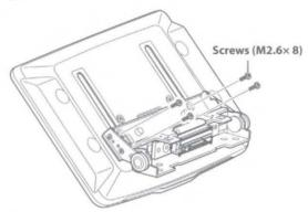
Attach the Sheet Rear in a position that aligns with the up-down position of the display unit.
