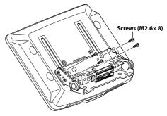
2 Attach the Sheet Rear in a position that aligns with the up-down position of the display unit.
