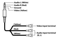
Configuration commercially available 4-pole mini AV plugs is not standardized.
