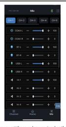
When you set the sound source signal on the PXE-C80-88/PXE-C60-60 main unit, it is divided into volumes for each output channel, the volumes of the respective sound sources on the channels are adjusted, and they are mixed.
