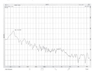
FFT spectrum analysis gives early clues to any audio distortion in the system. This distortion may occur through speakers being overloaded, amplifiers going into clipping, mixer signals overloading, and so on.
