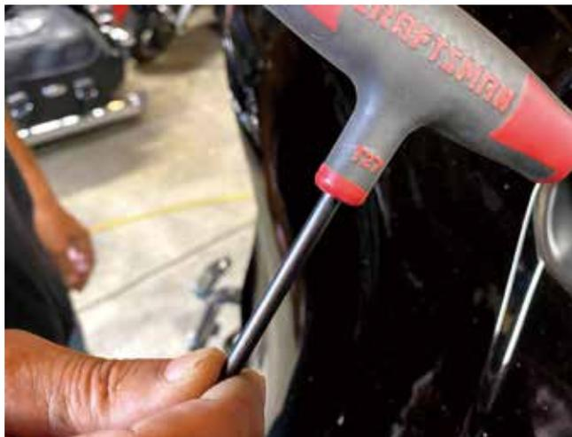
3. Remove (2) T-27 Torx bolts from outer edges of inner fairing near the fork tubes (facing forward)
