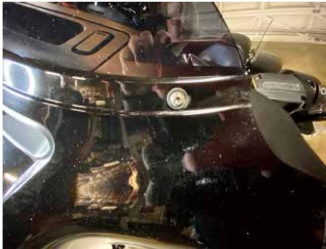
Note: Windshield and fairing will be loose once these screws are removed. Use extreme caution not to damage fairing or windshield. Lift away and unplug headlight to remove outer fairing.
