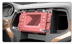
Remove the factory radio from the dash and disconnect the main wiring harness, antenna connections and USB from the back.
