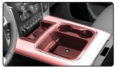
Reinstall the two (2) 7mm screws at the front of the center console.
