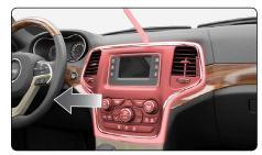
Disconnect the single wiring harness from the back.
