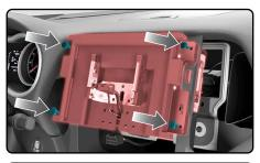
Press the FL-CH2 bracket and radio chassis into the dash cavity. Then, secure it with the four (4) Phillips screws removed earlier.
