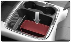
**13** Reinstall the rubber pad at the front of the center console.
