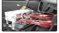
Make all connections to the back of the aftermarket radio (use head unit adapter OR cut connector from the FL-CH2 harness and connect the wires as shown in the wiring diagram). Make sure to connect the 4-pin data cable to the iDatalink I/F port and 3.5mm audio cable to the iDatalink I/F port.
