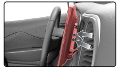
13. Slide the back cover in to place and secure it with the two (2) Phillips screws provided with the radio.
