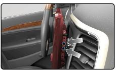
**12.** Slide the back cover in to place and secure it with the two (2) Phillips screws provided with the radio.
