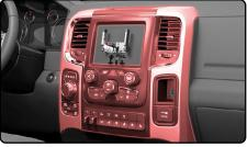
10. If applicable, reinstall the single (1) 7mm screw in the small pocket to the right of the radio controls.
