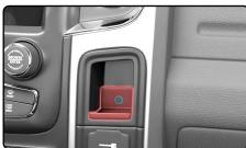
Secure the radio bezel with the two (2) 7mm screws removed earlier. Then reinstall the rubber pad.
