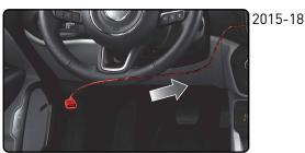
$\pmb{6B}_{\bullet}$  Connect the OBDII  $\pmb{c}$  cable to OBDII plug in vehicle. (2015-2018 only)
