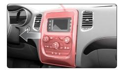
$\pmb{2.} \quad \text{Remove the four (4) 7mm screws securing the factory radio.} \\$
