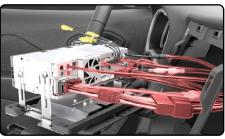
Press the FL-CH2 bracket and radio chassis into the dash cavity.
