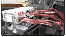
Press the FL-CH2 bracket and radio chassis into the dash cavity. Then, secure it with the four (4) Phillips screws removed earlier.
