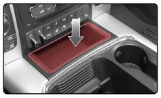
Reinstall the single (1) 7mm screw in the storage compartment.
