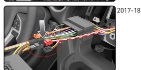
7. Press the FL-CH2 T-harness, Maestro module and antenna adapter into the radio dash cavity.
