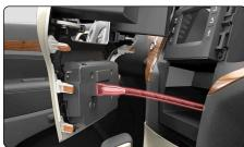
Remove the four (4) Phillips screws securing the radio into the dash.
