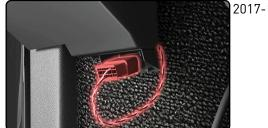
**6C.** Unplug 2-pin black connectors on main FL-CH2 harness. Connect OBDII **c** harness to main FL-CH2 T-harness. (2017-2018 only)
