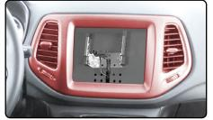
Snap the radio bezel back in place ensuring enough clearance with rubber pad, trim as necessary.
