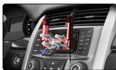
**15.** Connect the display cables to the back of the screen, routing them so they do not get pinched.
