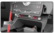
10. Carefully pull/pry outward on radio and climate control bezel to release the clips securing it in the dash. Disconnect and remove.
