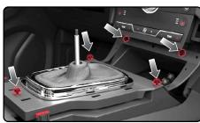
Disconnect and remove the shifter carriage.
