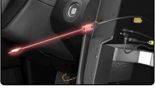
Locate suitable USB media hub replacement and route USB cables from pocket location to lower dash cavity (may differ from image).
