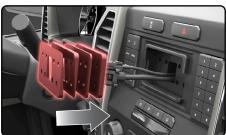
**15.** Mount the radio screen bracket onto the FL-F01 assembly, with supplied hardware.
