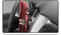
18. Slide the back cover into place and secure it with the two (2) Phillips screws provided with the radio.
