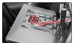
**17.** Secure the display to the bracket with the hardware supplied with the radio.
