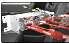
Make all connections to the back of the aftermarket radio (use head unit adapter OR cut connector from the FL-FO1 harness and connect the wires as shown in the wiring diagram). Make sure to connect the 4-pin data cable to the iDatalink I/F port and 3.5mm audio cable to the iDatalink I/F port.
