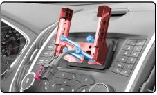
**14.** Connect the display cables to the back of the screen, routing them so they do not get pinched.
