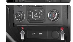
Remove the two (2) screws at the bottom of the radio and climate control bezel.
