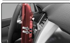
**16.** Slide the back cover into place and secure it with the two (2) Phillips screws provided with the radio.
