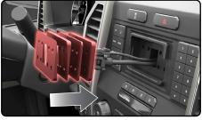
**14.** Mount the radio screen bracket onto the FL-F01 assembly, with supplied hardware.
