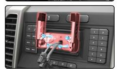
**16.** Connect the display cables to the back of the screen, routing them so they do not get pinched.
