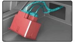
**12.** Remove the factory hub by releasing tabs with panel tool. Disconnect.
