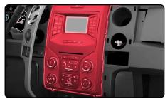
Disconnect and remove the radio and climate control bezel.
