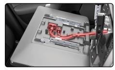
$\textbf{17.} \ \, \textbf{Secure the display to the bracket with the hardware supplied with the radio.}$
