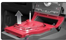
Move shifter back into PARK. Remove the two (2) 7mm screws at the base of radio bezel
