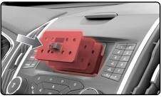
$\textbf{14.} \ \, \text{Mount the radio screen bracket onto the FL-F01 assembly, with supplied hardware.}$
