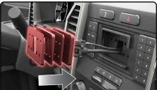
**15.** Mount the radio screen bracket onto the FL-F01 assembly, with supplied hardware.
