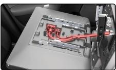
**15.** Secure the display to the bracket with the hardware supplied with the radio.
