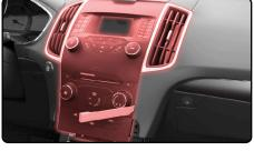
**12.** Remove the four (4) 7mm screws securing the radio display, then disconnect and remove.
