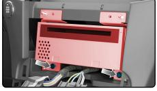
$\textbf{14.} \ \ \, \text{Factory USB hub need to be replaced with suitable USB media hub from FL-F01 dash kit.}$
