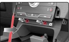
Carefully pull/pry outward on radio and climate control bezel to release the clips securing it in the dash. Disconnect and remove.
