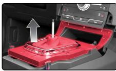
**10.** Move shifter back into PARK. Remove the two (2) 7mm screws at the base of radio bezel
