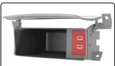
**15.** Remove the factory USB housing from the pocket by pressing the four (4) tabs using a small pick tool.
