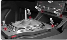
$\mathbf{R}_{\perp}$  Disconnect and remove the shifter carriage.
