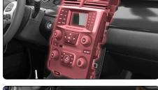
Remove the four (4) 7mm screws securing the radio display, then disconnect and remove.
