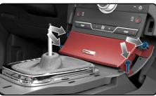
Remove the five (5) screw securing the shifter carriage.
