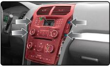
$\textbf{14.} \ \, \textbf{Use the provided plastic spacers to change the desired angle and depth of the display}.$
