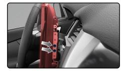
18. Slide the back cover into place and secure it with the two (2) Phillips screws provided with the radio.
