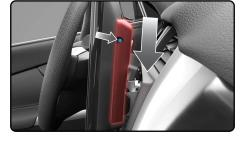
Put everything that was disassembled back into place, using reverse order of the removal steps.
