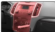
Remove the four (4) 7mm screws securing the radio display, then disconnect and remove.
