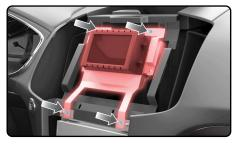
**12.** Remove the remaining two (2) 7mm screws at the bottom of the Audio control module/CD player. Disconnect and remove.
