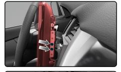
18. Slide the back cover into place and secure it with the two (2) Phillips screws provided with the radio.
