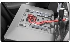
$\textbf{16.} \ \, \text{Secure the display to the bracket with the hardware supplied with the radio.}$
