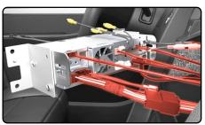
10. Press the radio chassis into the dash cavity and secure it with the two (2) 7mm screws removed earlier.
