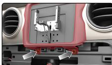
Reconnect the climate control panel and snap it into place.
