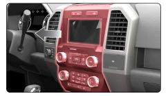
**6.** Remove the six (6) 7mm screws securing the 8" radio display, disconnect and remove.
