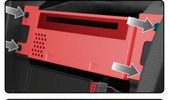
**6.** (If present) Remove the factory USB by pressing on the back the housing to release clips, disconnect and remove.
