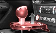
**8.** Using a panel tool, pry upward on the back of the center console to release the clips then slide backwards to release the front clips.
