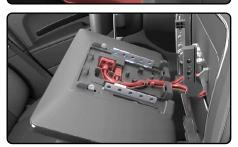
Secure the screen to the bracket with the hardware supplied with the radio.
