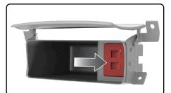
$11_{-}$  Remove the five (5) 7mm screws securing the shifter carriage.
