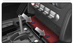
11. Open the Glove box and using the supplied panel tool, pry outward on the passenger side trim panel to the right of the compartment.
