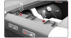
**5.** Carefully pull outward on radio and climate control bezel to release the clips securing it, disconnect and remove.
