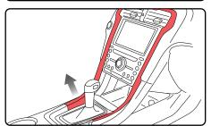
**5.** Remove two (2) 7mm screws holding the radio and control panel. Unclip, remove and unplug the radio and control panel.
