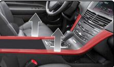
Remove the two (2) 7mm screws securing the shifter bezel then, from the bottom release the clips securing the boot to the shifter.
