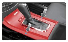
Remove the four (4) 7mm screws securing the radio hvac control panel, disconnect and remove.
