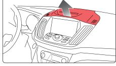
**?** Remove the two (2) 7mm screws from the radio bezel.
