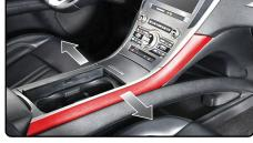
**2** Using panel tool release and remove the top center dash panel.
