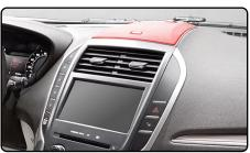
Remove four (4) 7mm bolts securing the radio fascia panel. Unplug and remove the panel.
