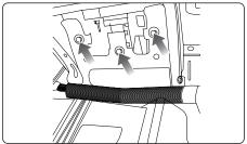
**3.** Without disconnecting the airbag, push it out far enough to expose the copper-plated 7mm screw on the left side of the airbag and extract it.
