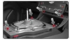
12. Remove the shifter carriage and disconnect the harness.
