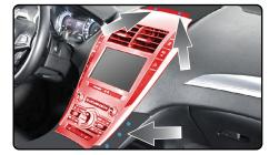
**6.** Remove the 2 bolts securing the CD player in the dash, disconnect and remove.
