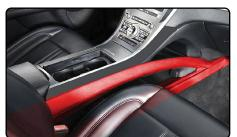
4. Open center console armrest lid and remove the four (4) bolts securing the trim/cup holder panel.
