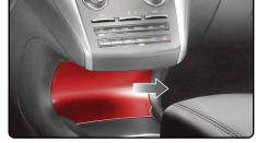
**?** Remove panel exposed, above previously removed panel.
