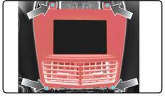
**8.** Remove four (4) 7mm screws holding radio screen into dash, disconnect and remove.
