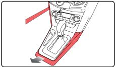
**3.** Remove three (3) phillips screws holding the shifter surround and climate controls.
