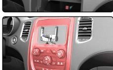
3. Connect the display cables to the back of the screen. Then, attach the black ground wire from the S8-F01 harness to the back of the screen using the single Phillips screw.
