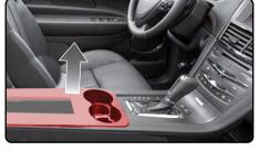
**?** Carefully remove left and right center console trim mouldings.
