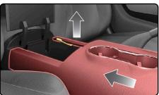
**Q** Remove tray pad below the radio to expose two (2) 7mm screws.
