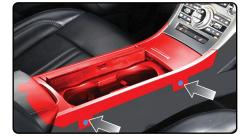
**5.** Remove eight (8) bolts securing the center dash/radio bezel in place. Disconnect and remove.
