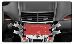
**6.** With a plastic panel tool carefully pry up the center top dash panel and remove.
