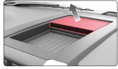
**2** Remove the two (2) 7mm screws securing the dash storage tray.
