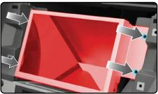
**9.** (If present) Remove the factory USB by pressing on the back the housing to release clips, disconnect and remove.
