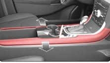
**2.** Engage the parking brake and place the shifter into the drive gear. Remove the upper console trim.
