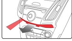
Remove the trim around the shifter console by prying it up and unclipping it.
