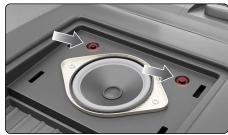
**3.** Using panel tool, release the clips securing the dash storage tray. If equipped, disconnect center speaker wire harness.
