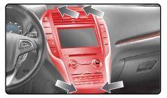
**5.** Remove two (2) 7 mm screws securing the CD player. Unplug and remove.
