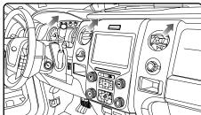
Remove two (2) 7mm screws from the top of the radio bezel.
