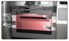
Remove Factory USB by pressing on the back the housing to release clips, disconnect and remove.
