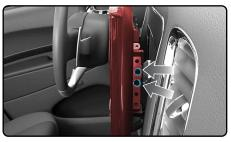
Slide the back cover in to place and secure it with the two (2) Phillips screws provided with the radio.
