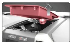
Remove the two (2) 7mm screws securing the radio and climate bezel.
