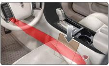
Pull the middle and rear of the side floor console lower trim panels (left and right) outward to release the retaining clips.
