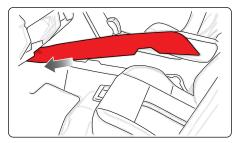
**10.** Position the front seats forward. Remove the two (2) rear floor console bolts.
