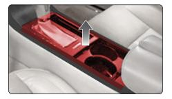
12. Remove the two (2) floor console to instrument panel bolts.
