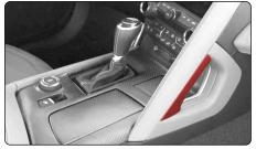
Remove side console trim panel by pulling out from the console.
