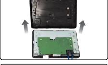
${\bf 27.}\,$  Cut the tab off the lower left of the back plastic bezel.
