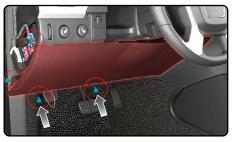
**24.** Reinstall the fuse box cover panel.
