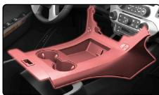
**21.** Reinstall the glove compartment rear panel and secure it with the three (3) T15 Torx screws. Make sure you pass the hanger through the designated hole in the panel.
