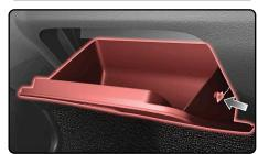
**23.** Reinstall the lower driver side panel and secure it with the four (4) T15 Torx screws.
