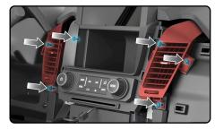
**17.** Reconnect the climate controls and snap the bezel back into the dash. Then, secure it with the two (2) 7mm screws.
