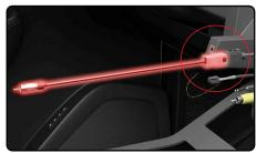
Route the USB cable supplied with the APX-S8-GM3, from the radio screen assembly to the glove box cavity.
