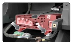
$\textbf{16.} \ \, \overset{\text{Open the glove compartment and disconnect the hanger on the right side.}}$
