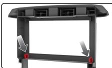
Flace the screen bezel onto the assembly.
