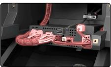
**15.** To remove the radio control module, press down on the 2 clips at the bottom of the module and slide the module out.
