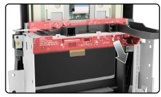
Remove the eight (8) gold T15 Torx screws securing the screen bezel and radio controls to the assembly.
