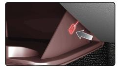
Press inward on the back of the compartment to release the retaining clips.
