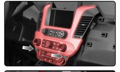
Reinstall the small dash panel to the left of the radio. If equipped with push to start, connect the wiring harness and secure it with the single (1) 7mm screw.
