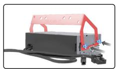
Place the S8-GM3-01 screen bracket into the assembly and secure it with the four (4) provided SM3-5P screws.
