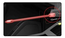
**7.** Route the USB-C cable provided to the center console, from the passenger kick area and remove the factory cables.
