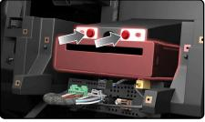
**14.** Disconnect the wiring harnesses, antenna connections and USB cables from the radio control module.
