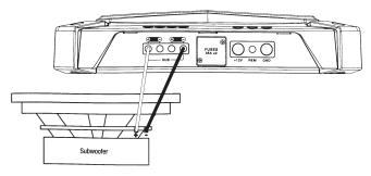
**NOTE:** Minimum speaker impedance for subwoofer operation is 2 ohms.
