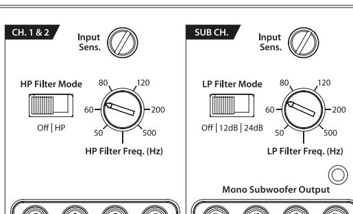
1) **“Filter Mode” Controls:** The M500/3 employs a 12dB per octave high-pass filter for its main channels. The Subwoofer Channel employs a low-pass filter with the option of 12dB or 24dB / octave slopes. Each of these filters can be controlled or defeated completely by way of the “Filter Mode” switch in each Channel Section:
