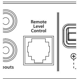
With the addition of the optional Remote Level Control (HD-RLC), you can control the volume of the subwoofer channel (Subwoofer Level) or of the entire M500/3 from a location of your choosing. This is useful for subwoofer level control, cabin speaker level control, zone volume control or even as a master volume control for the entire system.
