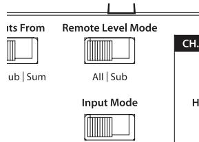
**Note:** In any of the three modes, the preamp output signal is not affected by any crossover filter selected (if the input signal is full-range, the preamp output will be full-range).
