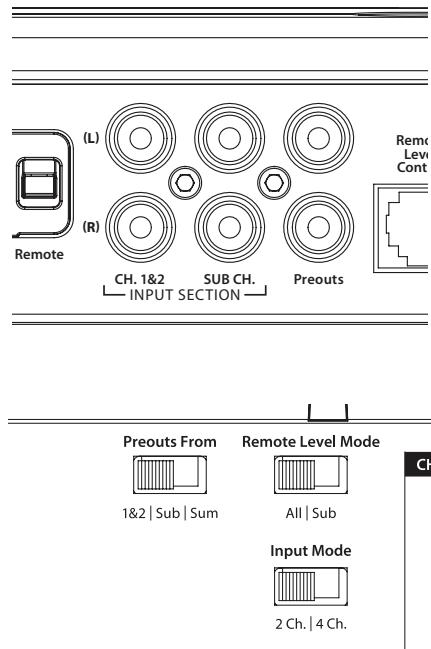
If you wish to send four discrete channels into the M500/3, simply use all four inputs and set the "Input Mode" switch in the "4 Ch." position. The amplifier will automatically combine the Sub Ch. input signals to mono.
