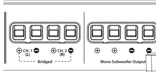
You will notice that there are two “+” positive connections and two “-” negative connections. This is to facilitate multiple subwoofer wiring. **The two positive and two negative connections are connected in parallel inside the amplifier** **They are not stereo outputs.** Connecting two subwoofers, each to one set of positive and negative terminals, will result in a parallel subwoofer connection. If only connecting one pair of subwoofer wires, it is not necessary to use both sets of connections.
