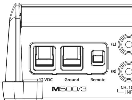
The M500/3's “+12 VDC” and “Ground” connections are designed to accept 4 AWG power wire. **4 AWG is the required wire size for this amplifier.**
