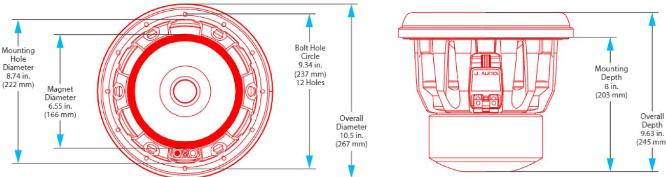
Net volumes given below do not include the air volume displaced by the speaker (Driver Displacement). This value must be added to the net volume along with the displacement of any braces and/or ports (if applicable) to arrive at a gross internal volume. Air inside a port is not part of the effective net volume. Calculate ports as solid, not hollow objects.
