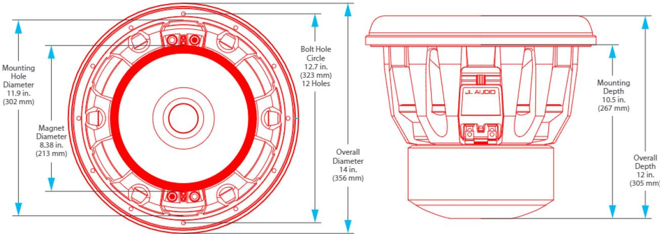
Net volumes given below do not include the air volume displaced by the speaker (Driver Displacement). This value must be added to the net volume along with the displacement of any braces and/or ports (if applicable) to arrive at a gross internal volume. Air inside a port is not part of the effective net volume. Calculate ports as solid, not hollow objects.
