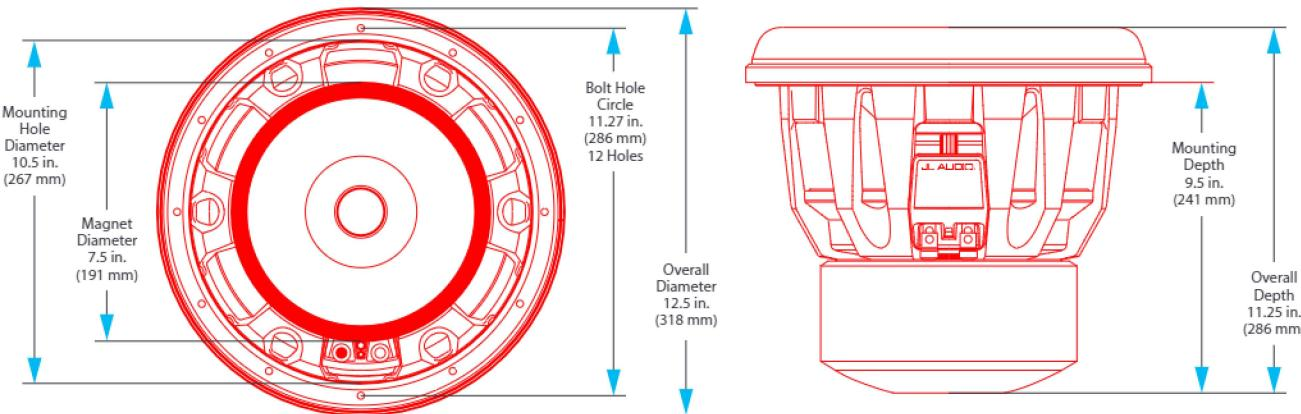
Net volumes given below do not include the air volume displaced by the speaker (Driver Displacement). This value must be added to the net volume along with the displacement of any braces and/or ports (if applicable) to arrive at a gross internal volume. Air inside a port is not part of the effective net volume. Calculate ports as solid, not hollow objects.
