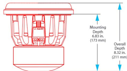
Net volumes given below do not include the air volume displaced by the speaker (Driver Displacement). This value must be added to the net volume along with the displacement of any braces and/or ports (if applicable) to arrive at a gross internal volume. Air inside a port is not part of the effective net volume. Calculate ports as solid, not hollow objects.
