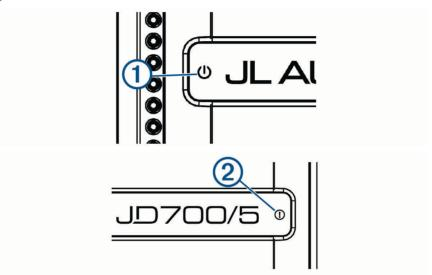
The power LED is solid blue when the amplifier is on.
