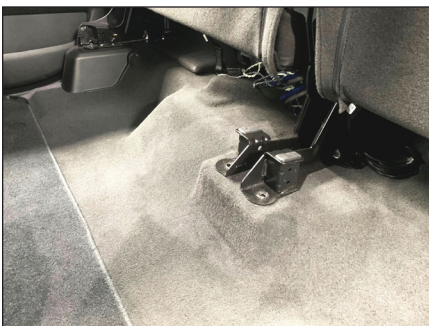
STEP 4 Using an E12 socket and wrench, remove the two inner seat bracket bolts.
