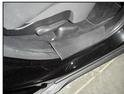
STEP 9 Remove the right rear door sill panel by carefully pulling up on the panel to release the clips.
