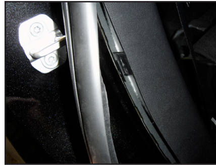
STEP 10 Pull the weather-stripping away from the side panel as shown, then unclip the side panel.
