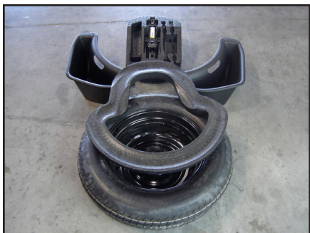
STEP 5 Remove the tool kit, the two storage pockets, the spare tire, and the padding from the tire well.
