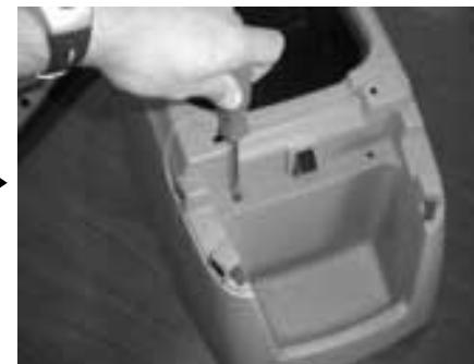
**STEP 10:** Install #8 x 1/2" black pan-head screws into the drilled holes.
