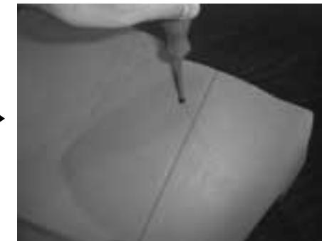
**STEP 8:** Install #8x 1/2" black pan-head screws into the drilled holes.
