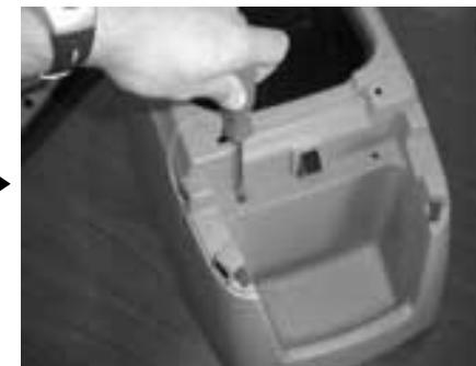
**STEP 12:** Remove the screws installed in **STEP 8** and **STEP 10**. Separate the console shell from the Stealthbox.
