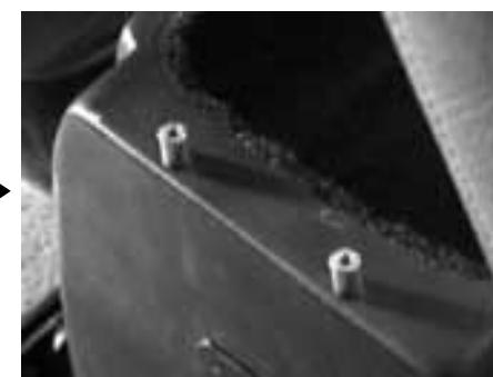
**STEP 26:** Connect the speaker wire to the terminal cup on the Stealthbox.
