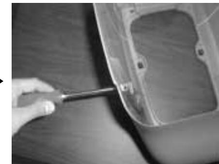
**STEP 5:** Reassemble the front and rear parts of the console shell using the supplied hardware (4 #8 x 1/2" long screws, 4 washers and 4 nuts) as shown in the picture.
