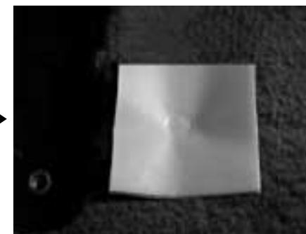
**STEP 16:** Using one of the supplied 3/8"x1-1/2" bolts, place the bolt through each hole of the front foot bracket (one at a time). Press down on the bolt, too leave impressions on the sheet wax squares.
