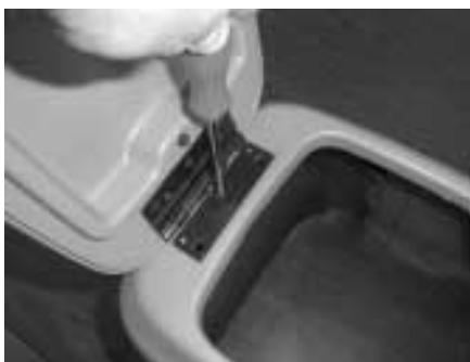
**STEP 13:** Attach the OEM's console lid to the shell. Use one of the OEM's screws and supplied speed-clip to the center hole of the hinge.
