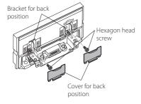
3 Pull the slider block forward and remove the two hexagon head screws to remove the bracket for back position.
