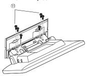
8 Attach the protective cover (accessory ②) to coupling part, and then fix it with two binding head screws (accessory ③).
