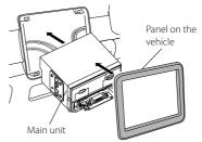
6 Install the display unit (accessory ®) to the main unit.
