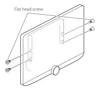
2 Adjust the display height according to the screw hole position. Default is "1".
