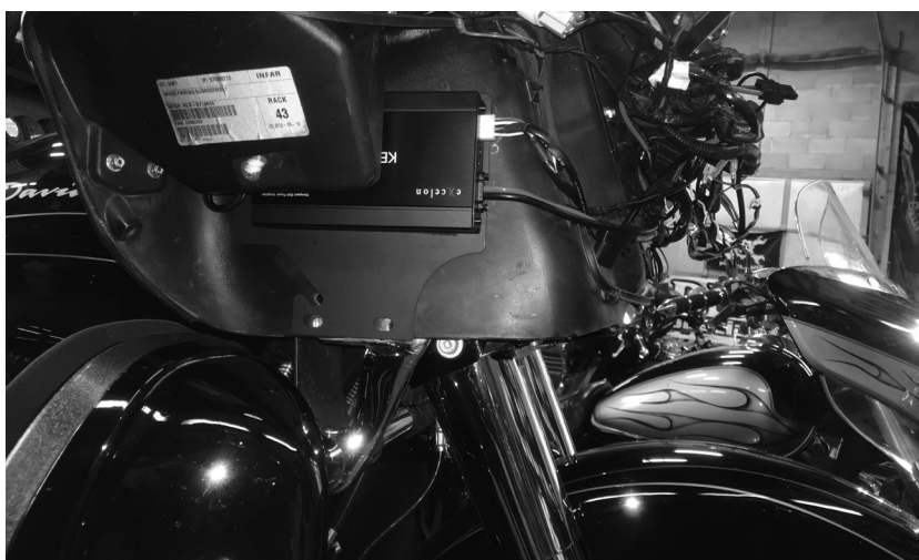
Fig 1.1 - Amplifier mounted to plate on bike
