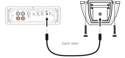
Remote cable passes audio; do not run cable parallel to power wires.
