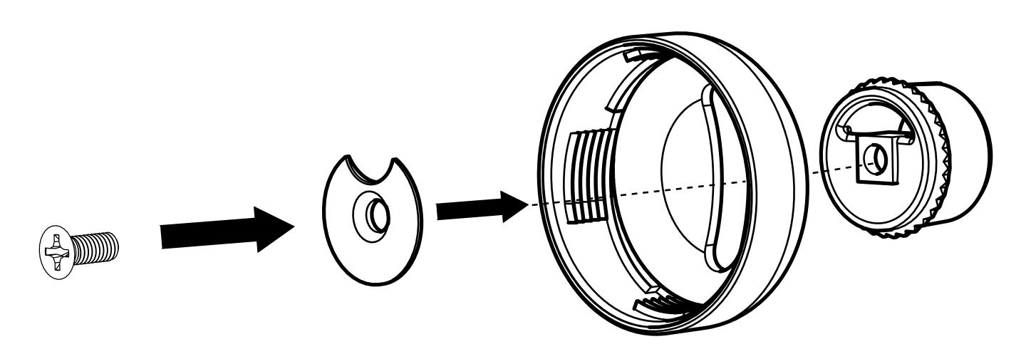
thread the tweeter wire through the washer, tweeter housing, and upper tweeter post \
