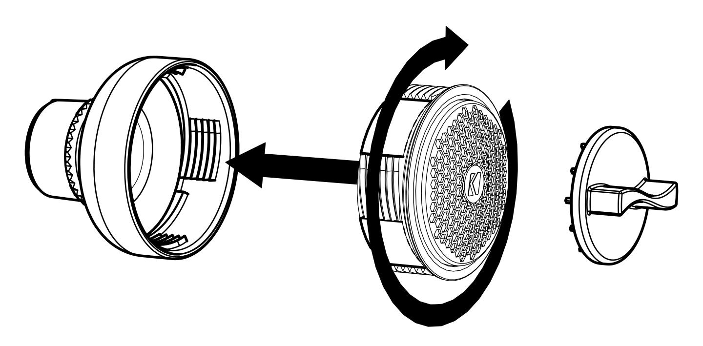
Thread the tweeter wire through the lower tweeter post and insert the tweeter assembly to the tweeter post until it clicks into place
