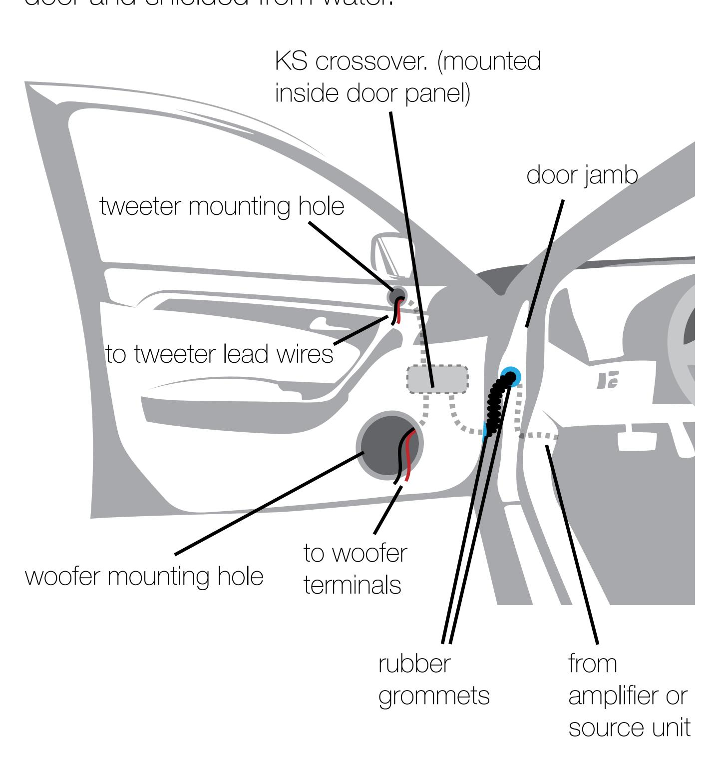
If factory speaker wiring is not available in your desired location, it may be necessary to run speaker wire through the door jamb. The speaker wire should be kept away from sharp edges and avoid the possibility of getting pinched by the door. An existing grommet in the door jamb is the ideal place to run the speaker wire. If the factory hole and grommet do not exist or are inaccessible, you must drill a hole to run the
