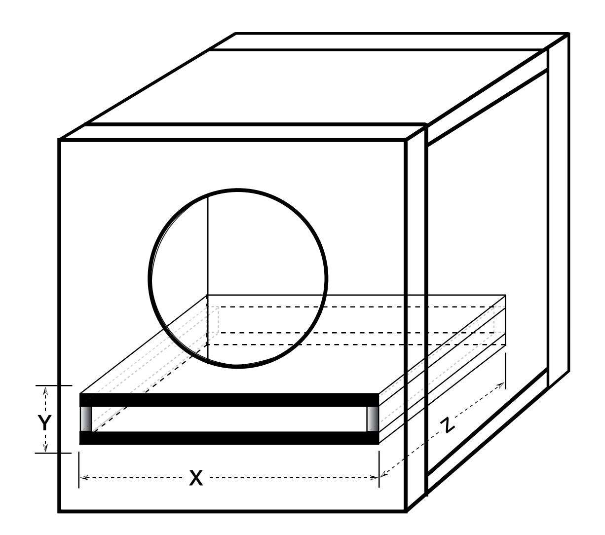
Do not install a port opening against a solid surface, such as an internal brace, backpanel or trunk wall, seat or interior panel of your vehicle. The port opening must remain unobstructed. Use the smallest dimension of the rectangular port as the minimum amount of space between the port opening and any solid surface to insure unrestricted airflow.
