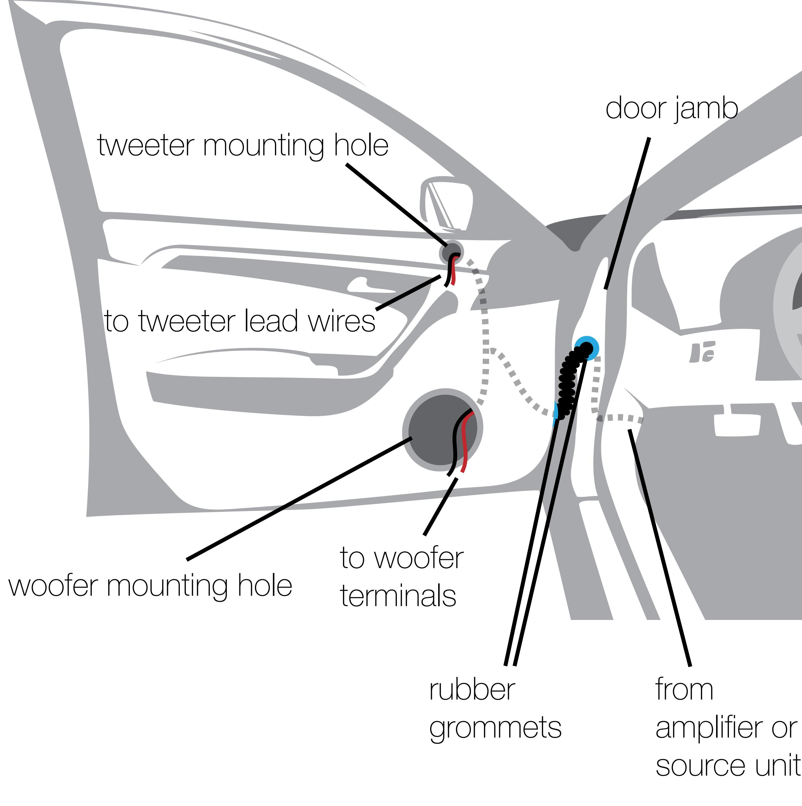
If factory speaker wiring is not available in your desired location, it may be necessary to run speaker wire through the door jamb. The speaker wire should be kept away from sharp edges and avoid the possibility of getting pinched by the door. An existing grommet in the door jamb is the ideal place to run the speaker wire. If the factory hole and grommet do not exist or are inaccessible, you must drill a hole to run the
