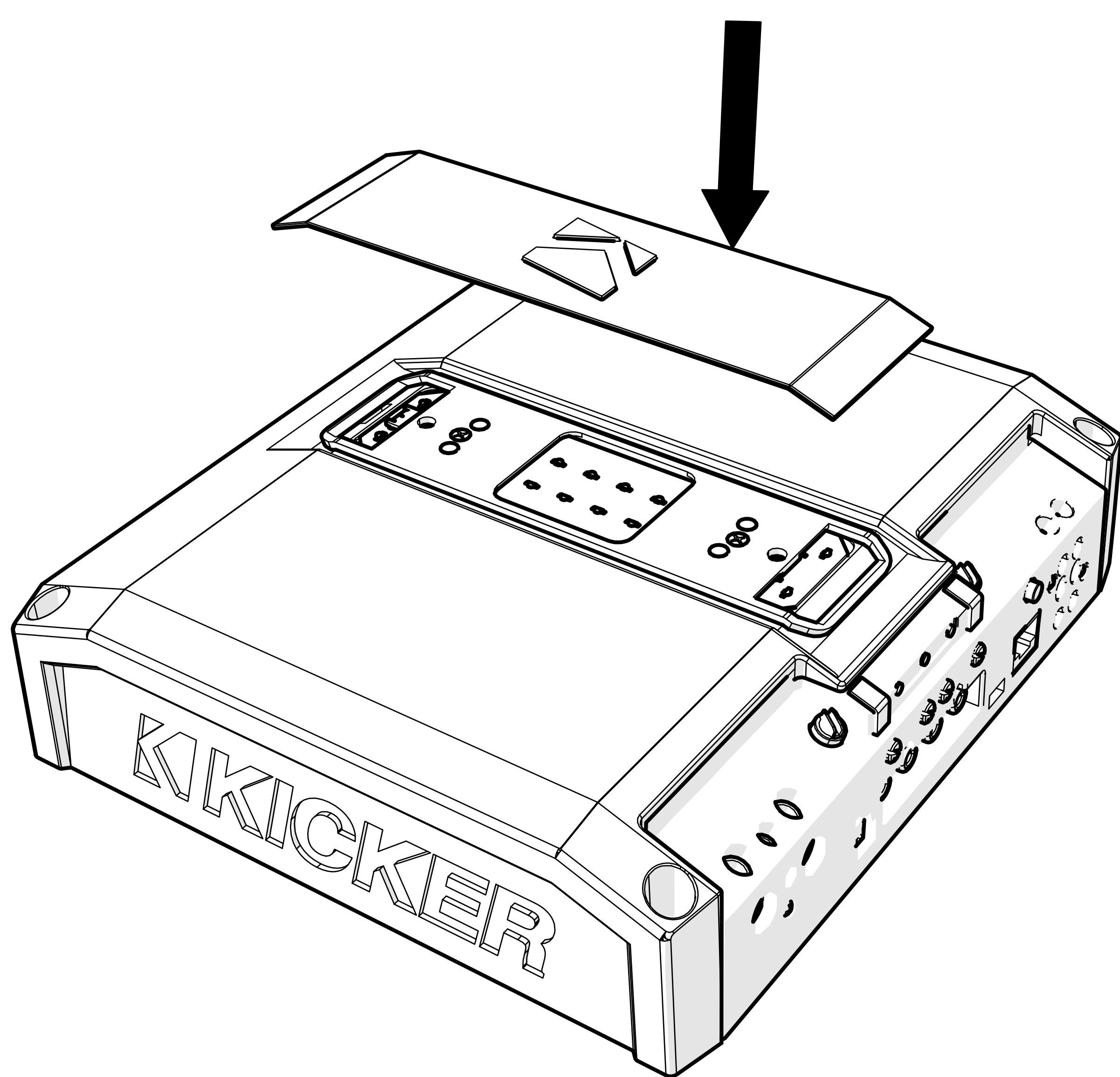
Remove the magnetized top panel cover to access the LX amplifier's power distribution and speaker output terminals, as well as gain and LED accent lighting settings.
