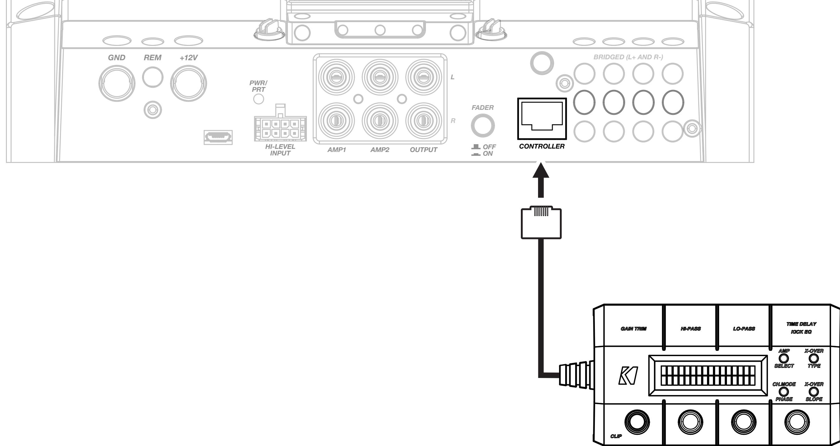
**GAIN TRIM:** Push the Gain Trim knob to open Gain Trim settings. Push the knob again or the Amp Select button to select the amplifier channel being modified. You can cut by -9dB or boost by +3dB per amplified section (AMP1 & AMP2). This allows you to make minor adjustments to levels, helping to match outputs, such as cutting your tweeter channels, while boosting the mids.
