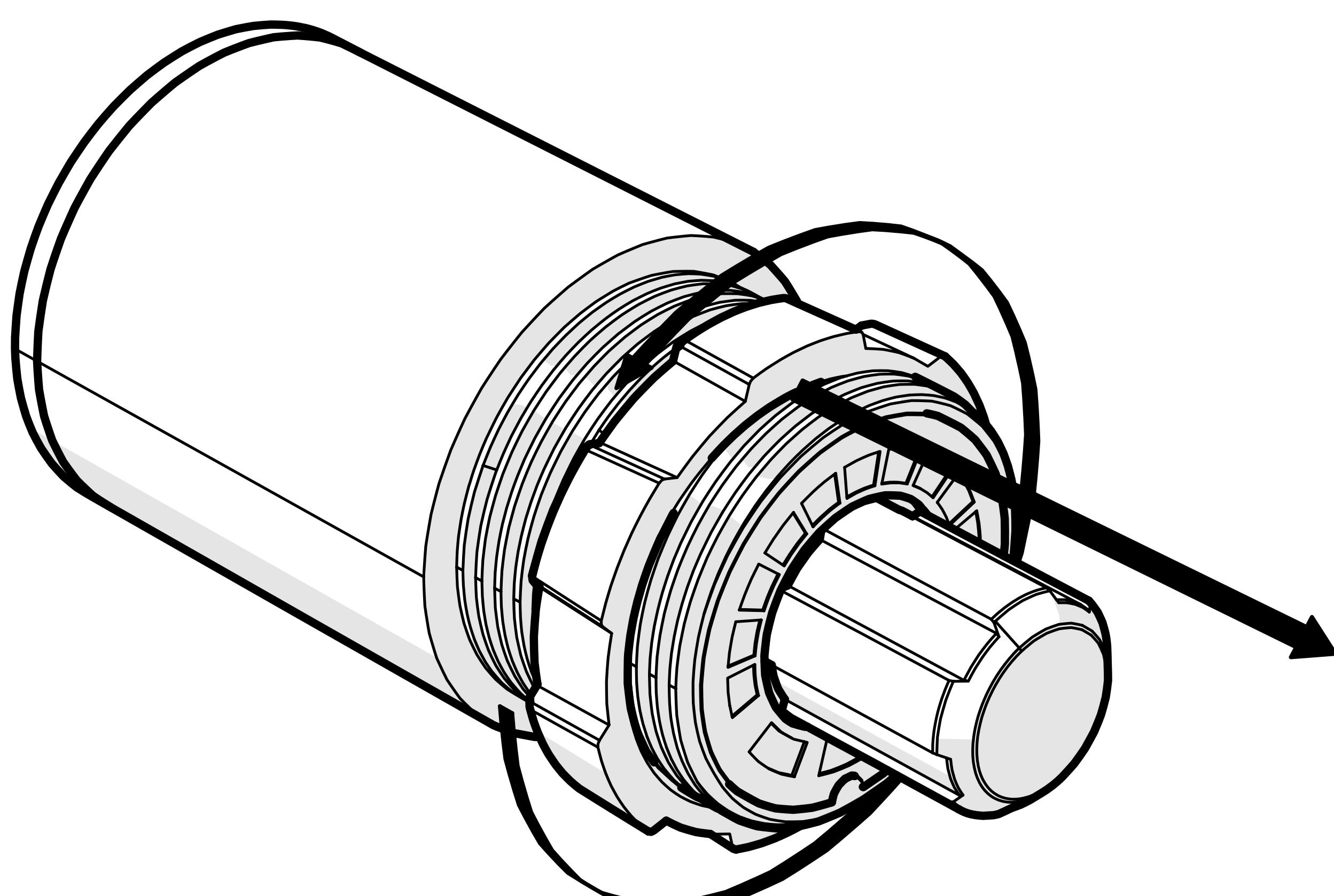
Place the LXRC through the mounting hole, then reattach the front mounting nut to secure the remote against the mounting surface.
