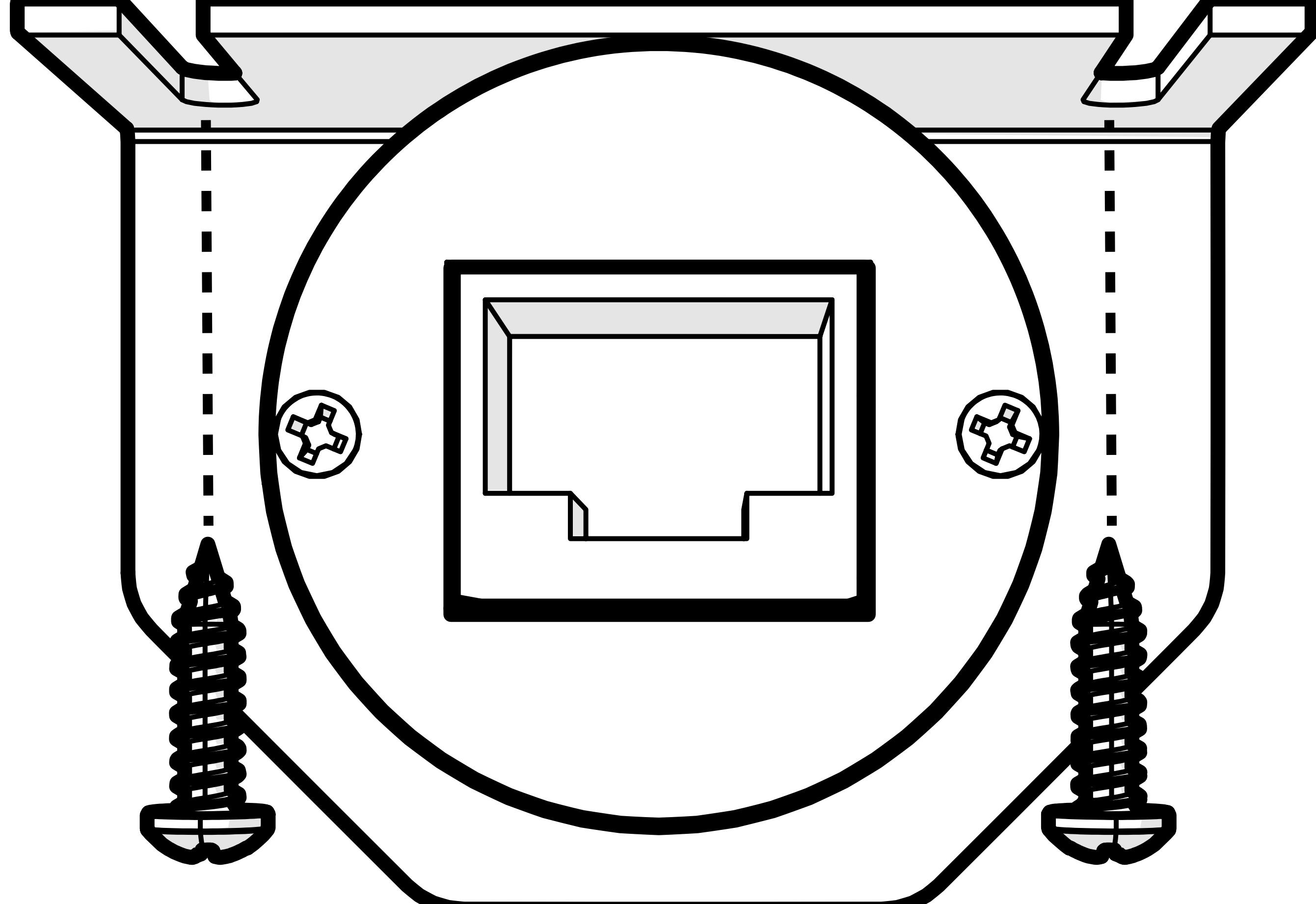
**Flush Mounting:** To flush mount the LXRC behind a mounting surface, begin by cutting a 1-inch diameter hole in the mounting surface, being careful not to drill through existing wiring or mechanisms.
