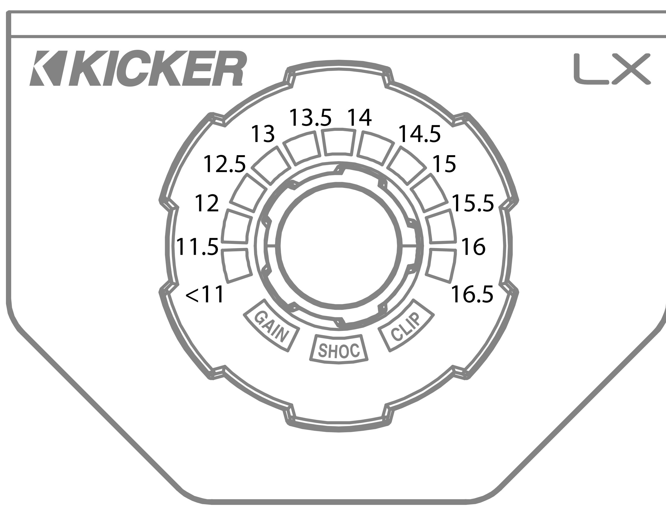
**Gain (Remote Level):** The LXRC gain control is a gain attenuator from -26dB to 0dB. This will allow you to conveniently adjust the gain of the subwoofer channel on the fly, with the maximum being the gain setting you've selected on the LX amplifier top panel. To enter Remote Level mode, turn the knob while in Voltage mode, or short-press the knob until the menu reaches Gain.
