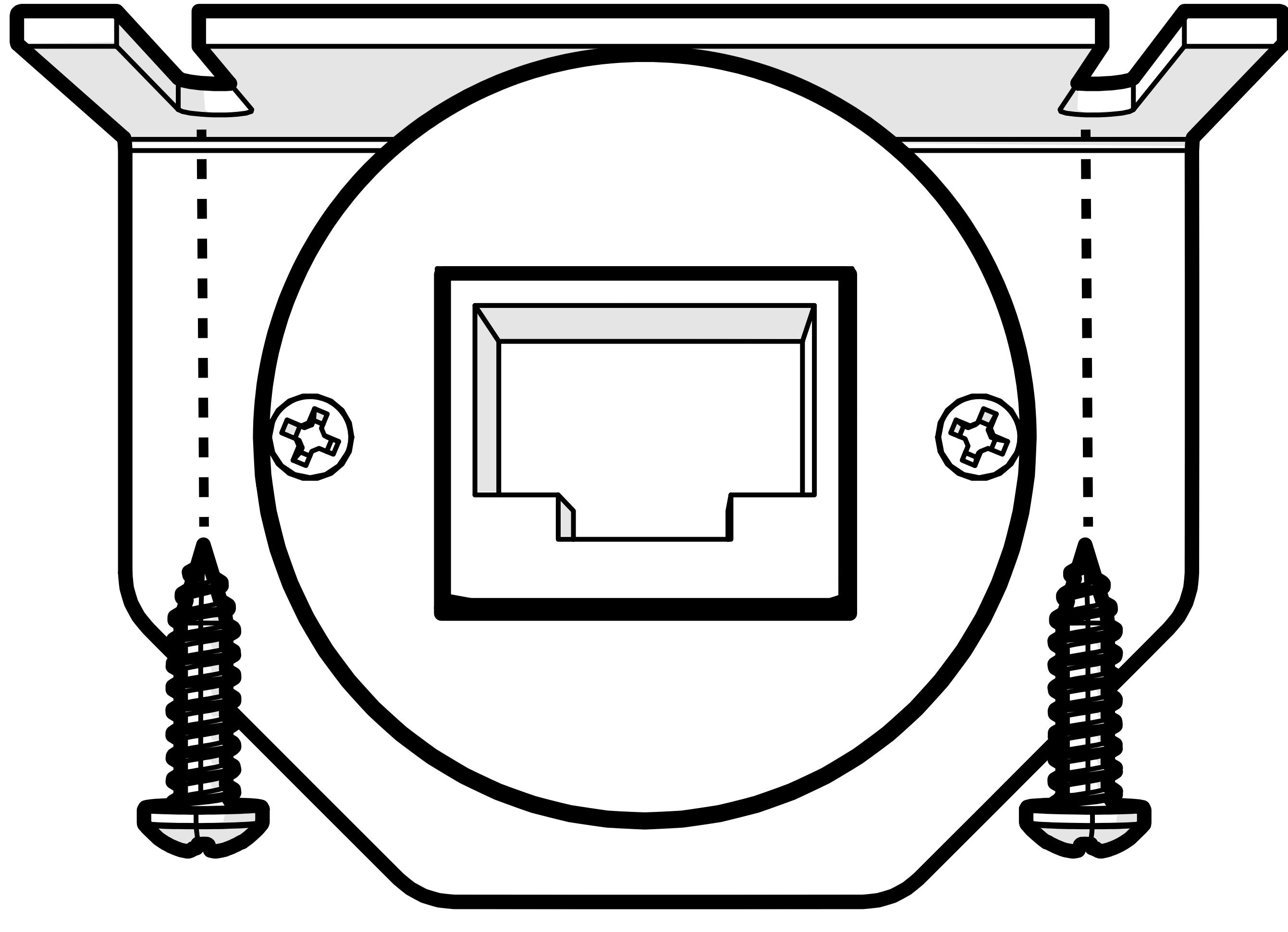
**Flush Mounting:** To flush mount the LXRC behind a mounting surface, begin by cutting a 1-inch diameter hole in the mounting surface, being careful not to drill through existing wiring or mechanisms.
