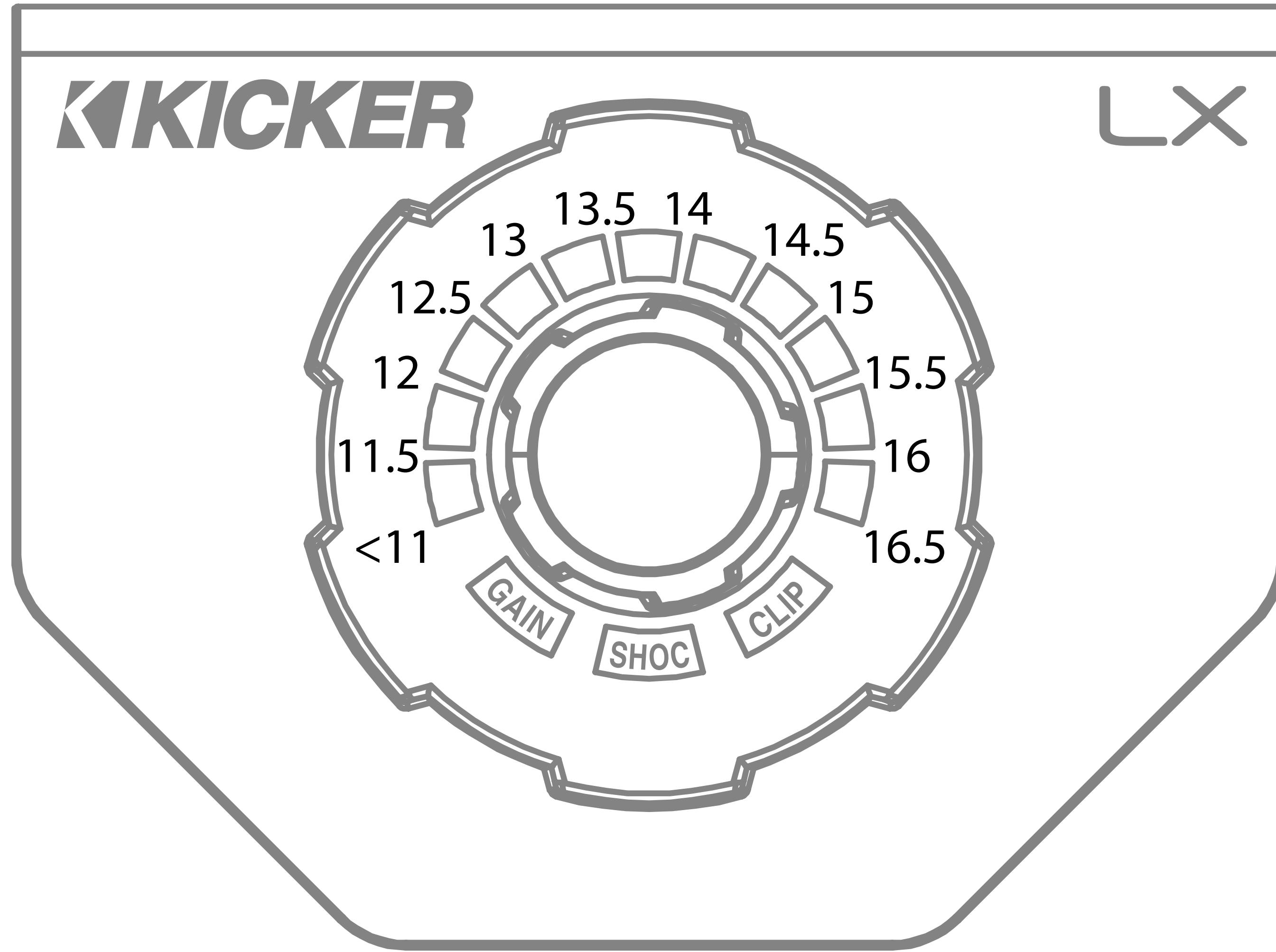
**Gain (Remote Level):** The LXRC gain control is a gain attenuator from -26dB to 0dB. This will allow you to conveniently adjust the gain of the subwoofer channel on the fly, with the maximum being the gain setting you've selected on the LX amplifier top panel. To enter Remote Level mode, turn the knob while in Voltage mode, or short-press the knob until the menu reaches Gain.
