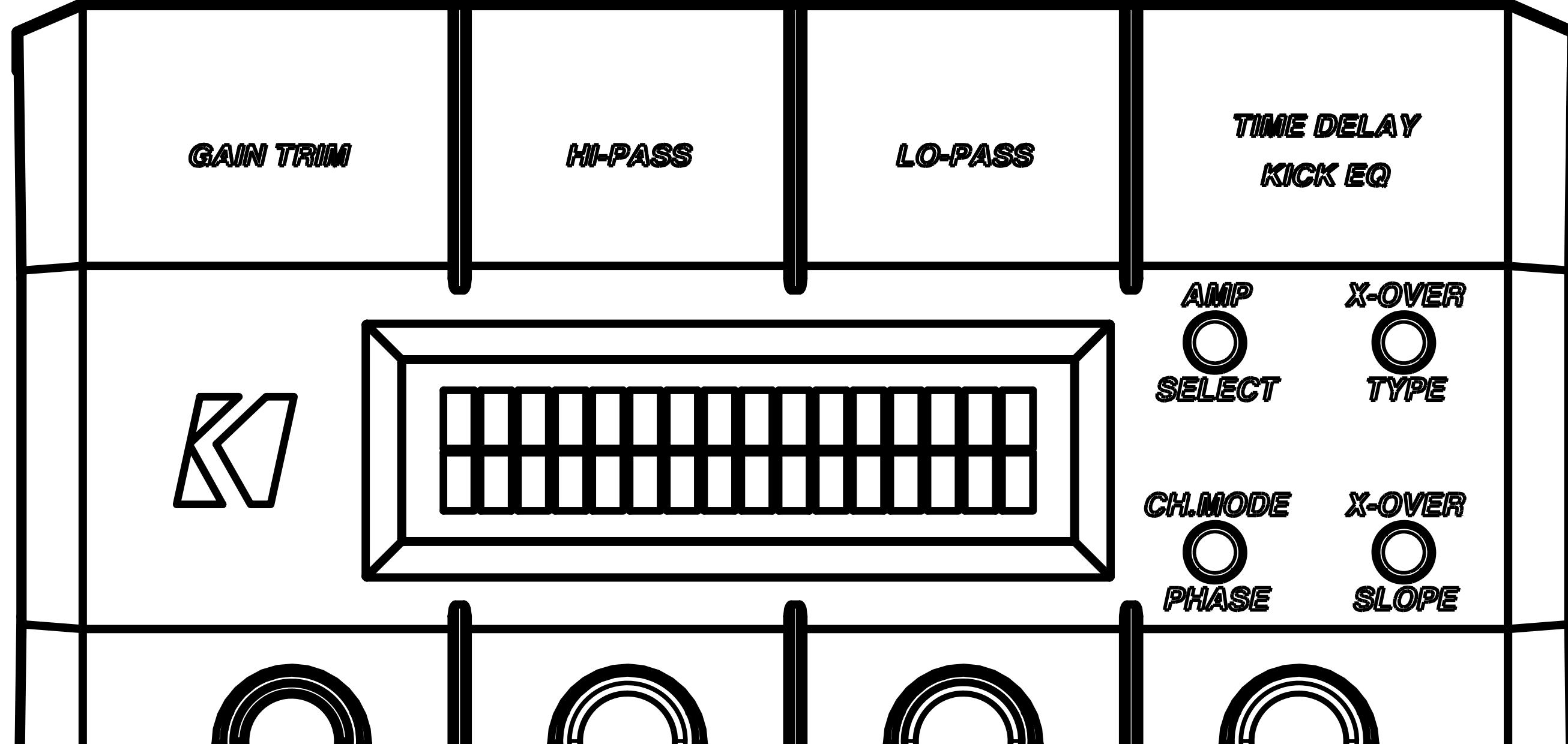
Once your LX amplifier has been installed, begin by connecting the RJ-45 cable of the LXCC to the Controller/Remote Bass input of the LX amplifier. The center display will immediately show real-time amplifier information, including amp model, amp temperature, and supplied voltage.
