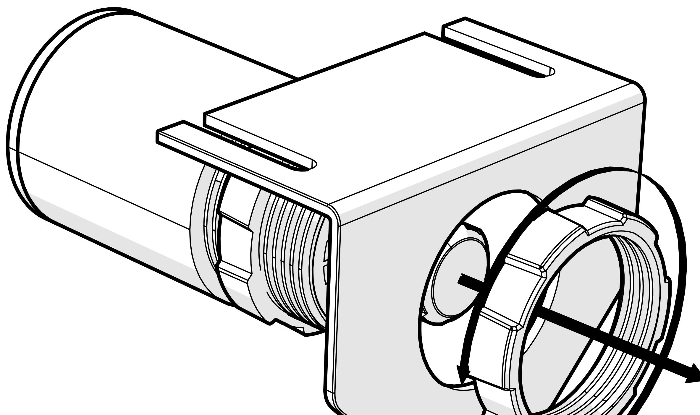
Adjust the rear mounting nut forward to set the protrusion of the LXRC knob.
