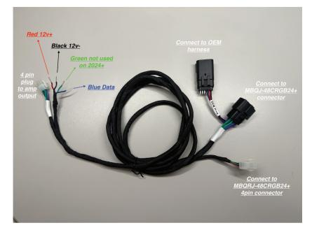
To the right is the the RGB wiring Harness diagram for the MBQJ-48CRGB24+ soundbar RGB wires when being used by itself without one of our stage kits.
