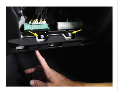
Once removed - pry off the piece surrounding the removed glove box and set it aside.
