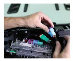
• Then plug the other ends of the green and blue harness into the slots on the back of the piece.
