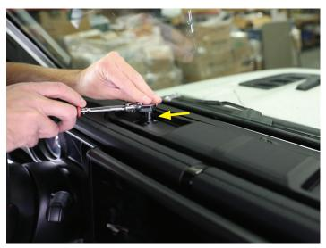
With screws removed, gently pry the piece out of place and set aside for now.
