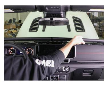
• Reinstall (2) 7mm screws at the top of the dash.
