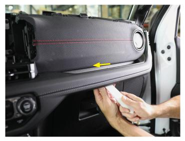
• Under the piece just removed, you'll have to remove (3) 7mm screws.
