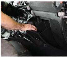
Once removed you'll need to remove another 7mm screw on the left-hand side of the glovebox.
