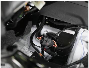
• Remove (4) 7mm screws holding in this piece in the back of the center console.
