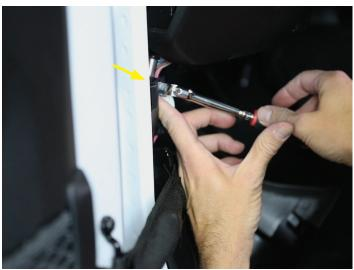
• Under the steering column, remove (3) 7mm screws.
