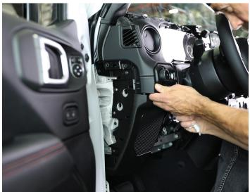
Remove (1) 8mm screw just to the left of the steering wheel. With that out, pry out this trim piece from the vehicle.
