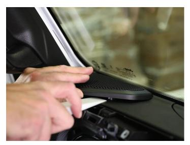
Remove the (2) 7mm screws holding the speaker in place. Repeat these steps on the passenger side of the vehicle.
