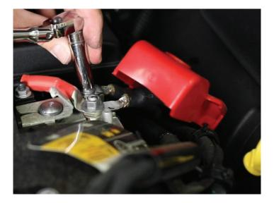
Place the fuse holder on the positive battery terminal and reinstall the previously removed nut. Then place the battery cover back into place.
