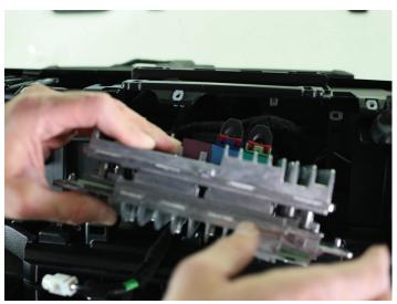
Disconnect the green and blue connectors. Plug in the green and blue harness provided in your kit into the connectors just removed.
