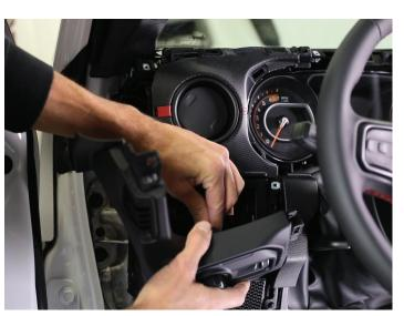
• Reinstall (2) 7mm screws just to the right of that piece. Snap it into place.
