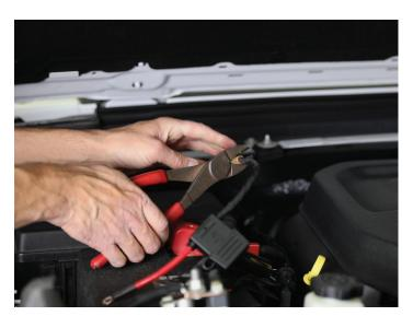
• Open the battery cover. Then disconnect the fuse from the fuse holder for now.
