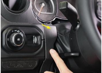
• Remove (4) 7mm screws on the top left of the dash.
