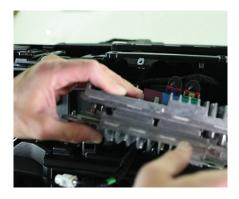
On the passenger side kick panel area, place the connector back into place and tighten down the previously removed bolt.
