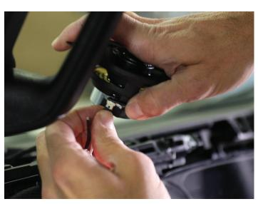
• Reinstall the (2) 7mm screws into place.
