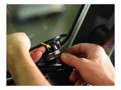
Back on the driver's side - remove the (4) 7mm to help gain access to the OEM speaker.
