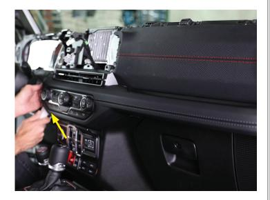
• Once removed-disconnect the two connectors and set it aside for now.
