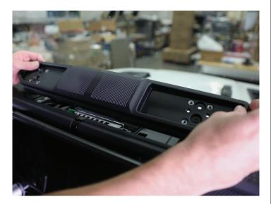
• Remove (2) 7mm screws underneath.
