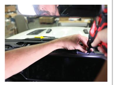
Once removed, gently pry off the monitor portion of the dash. After, flip it over and disconnect the two connectors and place it aside for now.
