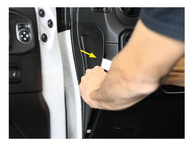
• Remove the piece under the steering wheel by gently pulling on it.
