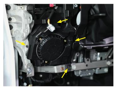
• Remove this 8mm bolt, these (2) 10mm bolts, and (1) 7mm screw.
