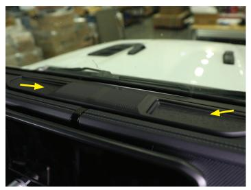
• Remove the (4) 7mm screws underneath. There are two on each side.
