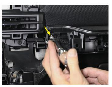
Plug the two connectors back into the long console piece and place it back into position.
