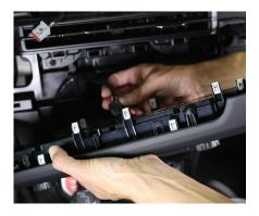
• Reinstall (3) 7mm screws on the backside of the grab bar.
