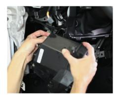
Remove (3) 7mm screws from the speaker and place the speaker off to the side.
