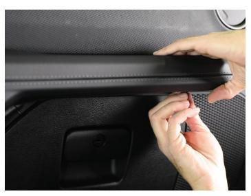
• Snap the piece back into position on the backside of the grab bar.
