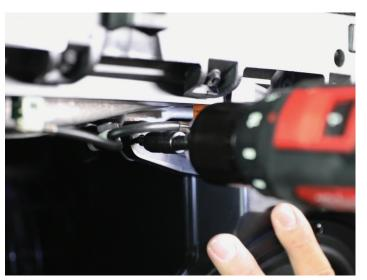
• Place the new speaker into position and reinstall the (2) 7mm screws to secure it to the vehicle.
