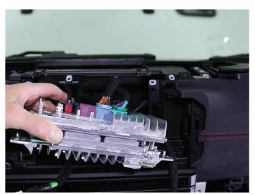
• Feed down the connectors into the back of the dash.
