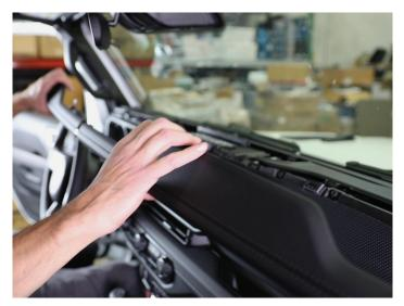
• Remove the (5) 7mm screws holding in the monitor portion of the dash.
