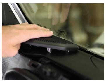
• Reinstall the front piece of the dash and press it into place.
