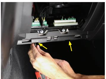
• Now we can reinstall the glove box and snap it back into place.
