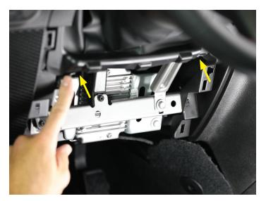
• After - install (2) 7mm screws and (2) 7mm screws a little lower.
