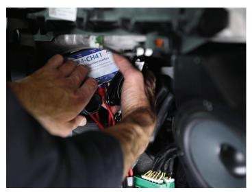
• Take your wiring and tuck into the center console underneath the floor mats all the way to the front passenger side seat.
