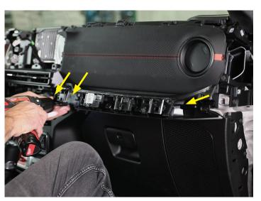
• Remove (3) 7mm screws on the right side of the glove box. After - open the glove box and remove it from the vehicle.
