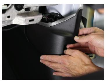
• Reinstall the piece surrounding the removed glove box.
