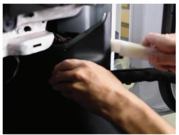
Remove this 10mm bolt and afterwards, use a trim tool to remove the connector.
