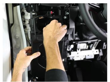
• Above that - plug in the connector on the lights knob and reinstall.
