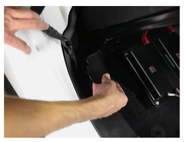
Place the seat back into its original position and reinstall the (4) E14 E-Torx bolts.
