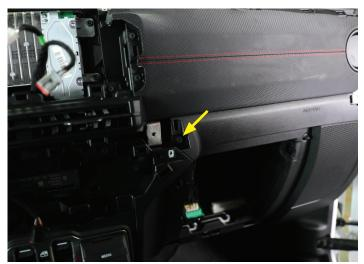
• After, remove (2) 7mm screws located at the bottom of the glove box.
