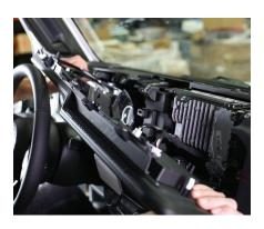
On the passenger side of the vehicle use a trim tool to pry off the backing on the handle above the glove box.
