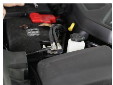
Reinstall the fuse into the fuse holder.
