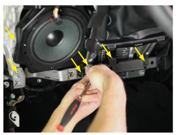
• Back up top - connect the wires to the new tweeter and place it into position.
