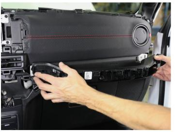
• Reinstall (2) 10mm screws holding in the back of the bar.
