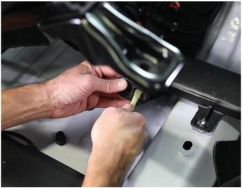
• Underneath the vehicle, route the power wire up to the engine bay. Following the OEM wiring.
