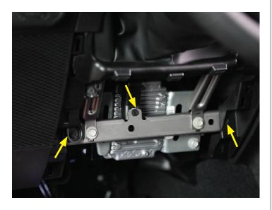
With those removed, wiggle out this piece to the left of the steering wheel and remove (2) 7mm screws underneath.
