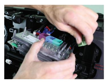
Plug in the green and blue harness provided in your kit into the connectors just removed.
