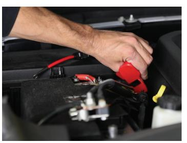
• Remove the 10mm nut from the positive battery terminal.
