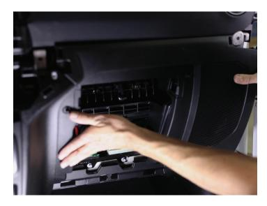
• Reinstall (2) 7mm screws underneath.
