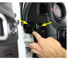
• Remove and disconnect trim with the lights switch.
