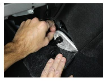
Back on the passenger side, route the speaker connector up through the glove box cavity to where the new speaker will go.
