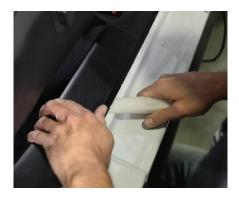
• Once free, run the speaker wire along and tuck it underneath the panel.
