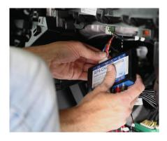
Prior to tucking away the PAC Module, set the dip switches on the PAC according to the provided PAC manual.
