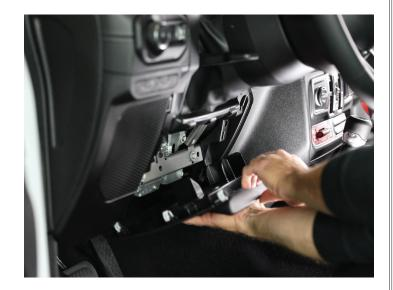
Bring over the center dash piece with the touch screen and reconnect the two connectors.
