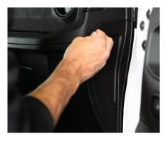
On the driver's side reinstall the speaker cover to the left of the steering wheel. Just above that, plug in the connector on the lights knob and reinstall.
