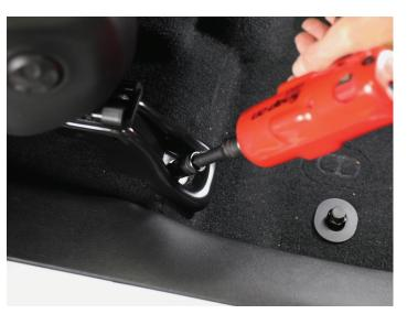
Lift up on the floor mats to gain access to this drain plug and remove it from the vehicle.
