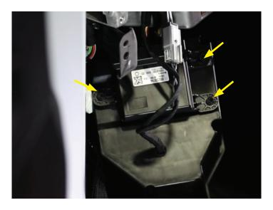
• Reinstall (2) 7mm screws above the speaker.
