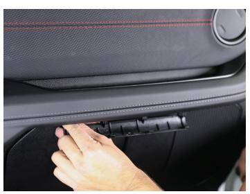
• Reinstall (3) 7mm screws as shown here. After - reinstall the trim panel.
