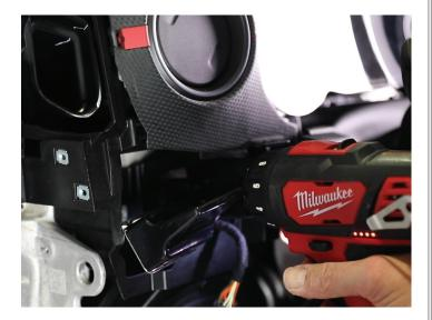
Insert an 8mm bolt, another 7mm screw, (2) 10mm bolts, and another 7mm screw.
