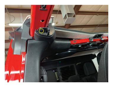
Unclip rear door sill panel first two clips by moving towards the center of the vehicle
