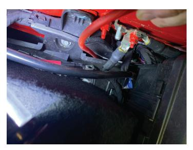
• Crimp and heat the fuse butt connector by the battery
