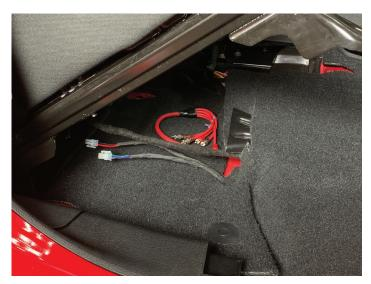
Connect the remote wire to the PAC Audio pigtail harness, then connect the interface box to the pigtail harness, (at this point the RCAs can be plugged in and reference the labels to connect properly)
