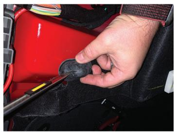
Pass the power wire through the grommet and to the underside of the vehicle, and then install the grommet back into its location
