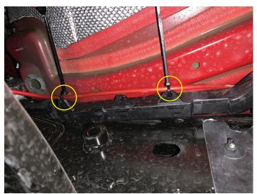
• Pass power wire up passenger fender near battery
