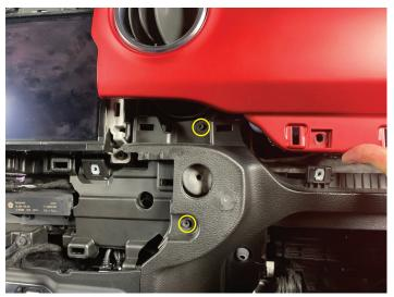
Remove (3) Phillips screws holding the passenger speaker enclosure, then disconnect wires and remove from vehicle
