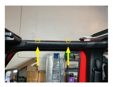
• Unclip and disconnect the dome light
