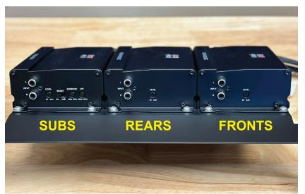
Tilting the passenger side seat forward, connect the power and speaker connections to the appropriate amplifiers. Amplifier position from previous step:
