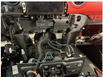
Disconnect large main harness connector on back of radio screen. Then connect the PAC Audio T-Harness into the radio and the OEM connector into the T-Harness. (for more information on the PAC Audio interface and wiring please refer to the instructions provided in the interface box)
