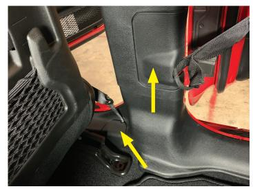
• Clip rear door seal panel into the B-Pillar panel
