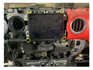
• Unclip lower center console and move toward rear of vehicle
