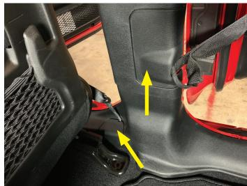
• Unclip and remove B-Pillar sill panel
