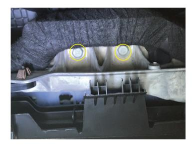
Carefully unclip the air bag. (this does NOT need to be removed from the vehicle)
