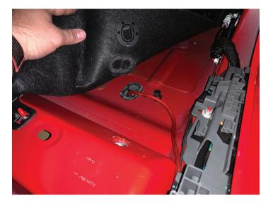
Under the vehicle zip tie the harness along the OEM wire channel should move forward into the fender area
