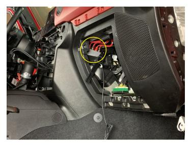
Place amplifier power connections under passenger seat routing power wire along OEM wiring toward floor grommet (Also connect the remote wire at this time)
