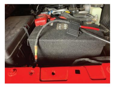
Remove 70A MAXI fuse and make connection to the battery with a 10mm socket
