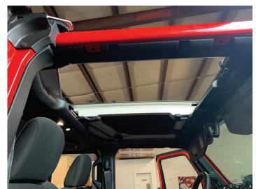
Remove (4) T25 Torx screws from the passenger side upper roll cage cover and set aside
