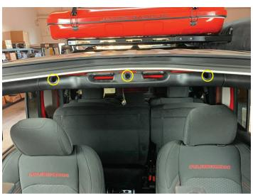
Remove the fir tree clip, then gently unclip the T-panel, (you will NOT be removing from the vehicle just gaining enough space to pass soundbar wiring behind)
