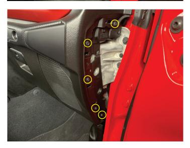
Using a panel tool carefully remove the grab handle cover (starting on the left)
