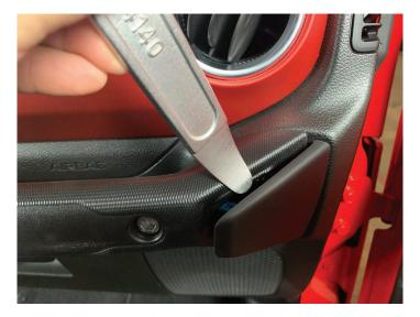
Remove (2) 10mm bolts securing the grab handle and set handle aside
