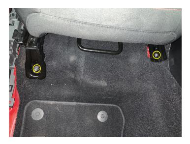
Slide passenger seat forward and remove (2) T-50 Torx bolts from the rear
