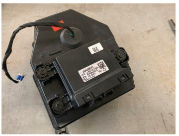
Install the module on the new enclosure using the OEM hardware and install the speaker pod back into the dash.
