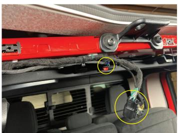
• Clip the T-panel into place and install the first tree clip
