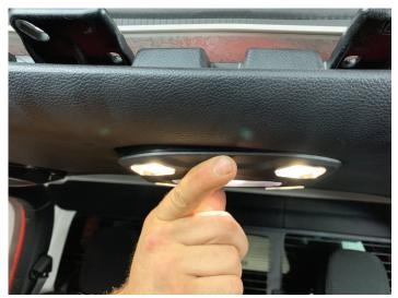
Place passenger roll cage cover into position and install (4) T25 Torx screws
