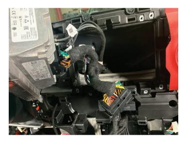
Route T-Harness pigtail from radio pocket to lower console behind metal brace
