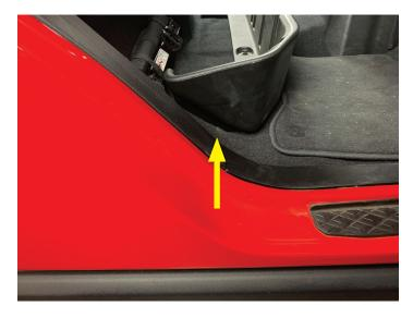
Unclip the two covers on B-Pillar sill panel
