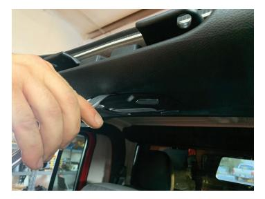
Remove (3) T-25 Torx screws from the front edge of the soundbar cover and then unclip and remove set aside
