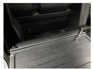
• Remove (2) bolts on driver side rear panel using a 10mm ratchet. Then remove from vehicle.
