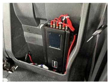
Fish excess wiring back into the hole in the bottom of the pocket.
