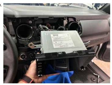
• For vehicles 2017 to 2019 with no factory amplifier. You will be using this harness behind the radio. If you have the OEM radio then connect the LOC module to the harness. If you have an aftermarket headunit you will not use the LOC.
