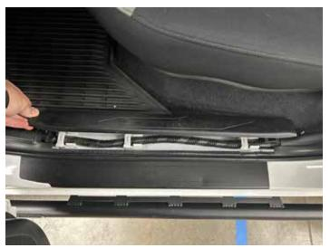
• Unclip the sides of the driver seat belt cover. Then remove the (1) 14mm bolt.
