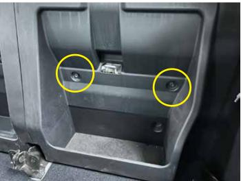
Remove (2 or 3) bolts on passenger side rear panel using a 10mm ratchet depending on vehicle trim. Then remove from Vehicle.
