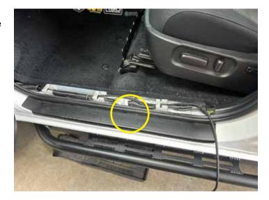
Route the power wire under the B Pillar moving toward the driver side rear sill area.
