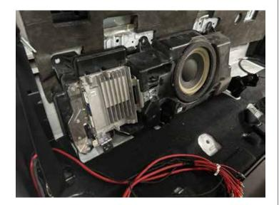
• Connect the short pig tail harness to the OEM amplifier T-harness.
