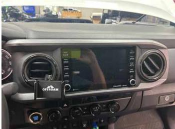
• Remove (4) 10mm bolts holding the radio to the dash.
