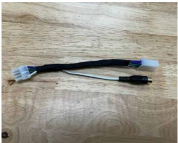
If you have the OEM headunit and is factory amplified you will install the correct PAC Audio interface behind the radio.
