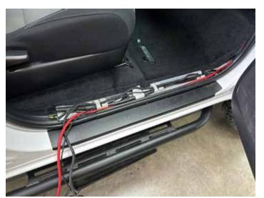
Route the harnesses down the passenger rear door sill along the OEM harnessing and continuing toward the vehicles rear wall.
