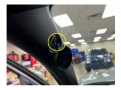
Pull out on the top of the A-pillar and then pull back toward the rear of the vehicle to remove the panel.
