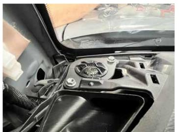
• Remove the door window trim by carefully prying with a panel tool.
