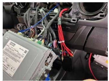
Connect the blue remote wire to the T-Harness, PAC module or aftermarket headunit. Then pass from the radio area to the passenger floor area. On '20 – '23 non-JBL amplified vehicles, you will not connect the REM wire.
