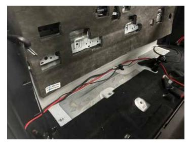
Connect the short pig tail harness to the speaker extension harness and continue routing to the driver side.
