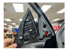
• Carefully push in the center of the push pin to release the clip and remove.
