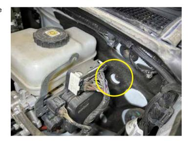
On the inside driver side firewall near the brake pedal support, cut the matting where marked by the yellow dashed lines using a utility knife.
