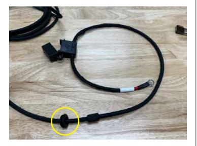
Pass the power wire through the firewall and install the grommet.
