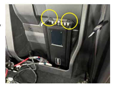
Connect the RCAs to the amplifier in the following order: Front Black RCA to Channel 1 Front Red RCA to Channel 2 Rear Black RCA to Channel 3 Rear Red RCA to Channel 4 Sub Black RCA to Channel 5 Sub Red RCA to Channel 5
