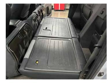
• Using a panel tool remove the (2) covers on the driver side rear seat back.
