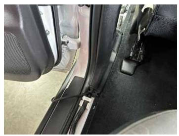
Route the power wire down the driver side rear wire channel along the OEM harnessing toward the rear cabin wall.
