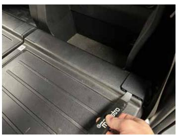
Using a 14mm ratchet, remove (2) bolts from the driver side rear seat back.
