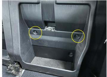
Remove (2 or 3) bolts on passenger side rear panel using a 10mm ratchet depending on vehicle trim. Then unclip back panel from wall and remove from vehicle.
