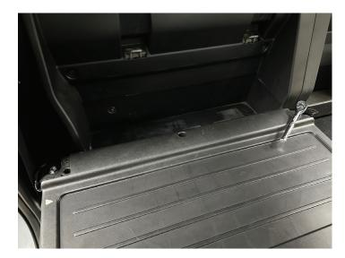
Remove (2) bolts on driver side rear panel using a 10mm ratchet.
