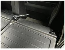
On passenger side rear seat remove (1) bolt from the middle seat belt with a 14mm ratchet.
