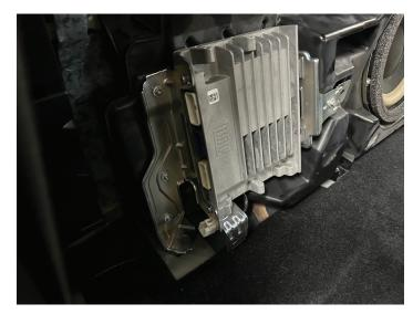
RRemove (2) bolts with a 10mm ratchet securing the OEM subwoofer enclosure. Then remove from vehicle.
