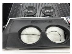
• Apply foam gasket tape along top edge of enclosure.
