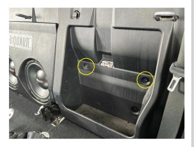
Using a 1/8" drill bit, drill (4) holes into the sub enclosure through the previous drilled holes on the driver side rear panel.
