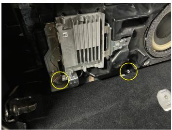
Remove (4) T20 Torx screws holding the OEM amplifier to the OEM subwoofer enclosure.
