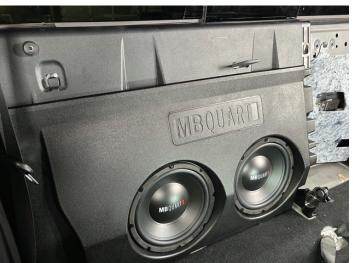
Install driver rear panel back into the vehicle and install (2) bolts with a 10mm ratchet.
