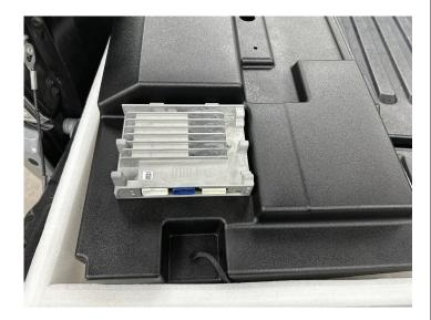
• Alnstall (2) M6 speed clips at the positions shown.
