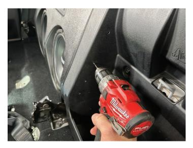
Install (4) ST4.8 x 32mm Torx screws and (4) M5 washers using a T20 Torx.
