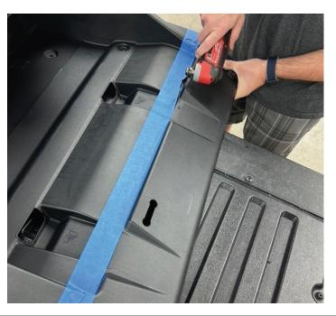
Remove (8) ST4.2x19mm Torx screws holding the subs to the enclosure using a T20 Torx. Then set subs aside for installation in a later step.
