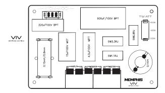
VIV35CV2 Crossovers uses switches to adjust a variety of features allowing the user to dial in the perfect sound for their audio system.
