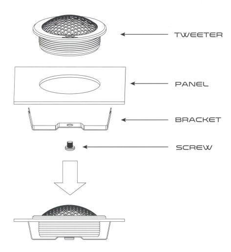
Tweeters should be positioned high, preferably at ear level. Optimum performance will be obtained when tweeters are angled toward the listener
