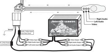
**Note:** This cable is intended for use in conjunction with an OS-4 to retain all safety and convenience systems. The vehicle should be equipped with a Panasonic Overhead LCD and IR system, in which the DVD player was part of the AM/FM/CD receiver. The OS-4 is needed to power the IR headphone system.
