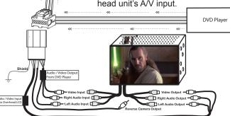
Note: This cable is intended for use in conjunction with a C2R-CHY4 (Rev 1.1.4 or higher) to retain all safety and convenience systems. The vehicle should be equipped with a factory Overhead LCD and IR system, in which the DVD player was either part of the AM/FM/CD receiver or a seperate stand alone unit.
