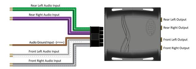
**Note:** If using large RCA connectors that are difficult to insert into housing, unsnap the L.O.C.PRO™ cover and remove end panel insert around RCA outputs.
