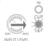
Adjust the Input Level knob until the Output Clip Indicator illuminates to the appropriate color. Repeat for all channel levels of input.
