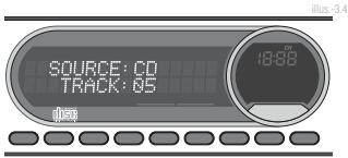
Note: Use the 40Hz @ 0dB tone (Track 5) for mono amplifier applications or the 1kHz @ 0dB tone (Track 7) for multi-channel amplifier applications. Be sure your x-over is switched to the appropriate filter setting.
