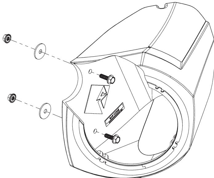
Step 3. Mark for the three holes to be drilled, remove the enclosure and drill.
