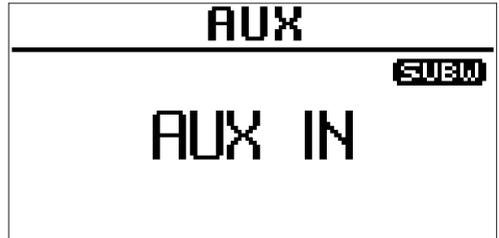
After your device is plugged into the source unit, this feature allows you to play music from your device. Select the AUX source option on the source unit and use your plugged in device to control song/track selection, PLAY/PAUSE and track skip FWD/REV.
