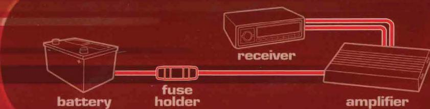
Includes power & ground wires, signal cable, MAXI fuse holder w/100 amp fuse, turn-on lead, ring terminals & hardware
