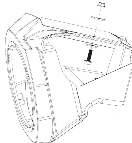
Step 3. Secure the enclosure using supplied hardware.
