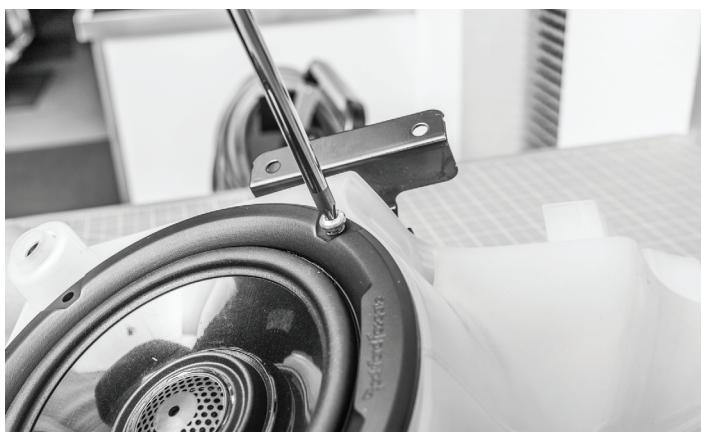
Secure the speaker to the factory pod using the factory hardware.
