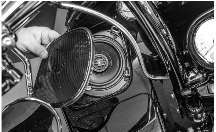
Reattach the pod with the factory hardware and reinstall any wire harnesses that were removed for the pod removal.
