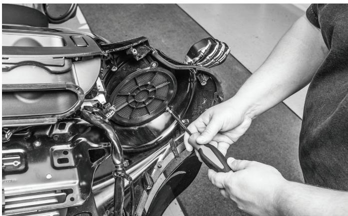
Using a screwdriver, remove the speaker grille that is attached to the fairing.
