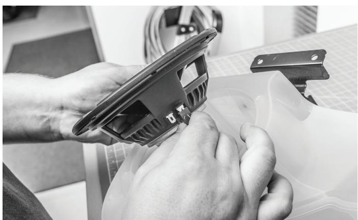
With the pod on a bench, unscrew the mounting screws to remove the factory speaker from the factory pod.
