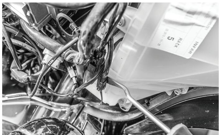
There are several wire connectors that are attached to the speaker pods and surrounding components that will need to be removed prior to unbolting allowing access to the bolts holding the pods in place.
