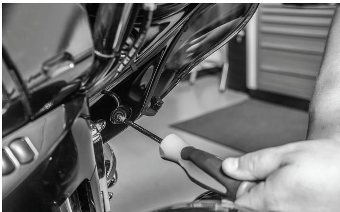
Once you have the windshield set aside, remove the remaining screws on the inside of the fairing.
