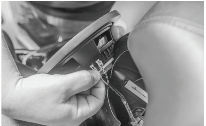
Connect the speakers by sliding the speaker wire connector over the speaker terminals
