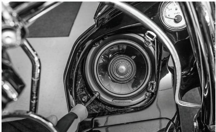
Secure the speaker to the pod using the factory hardware.
