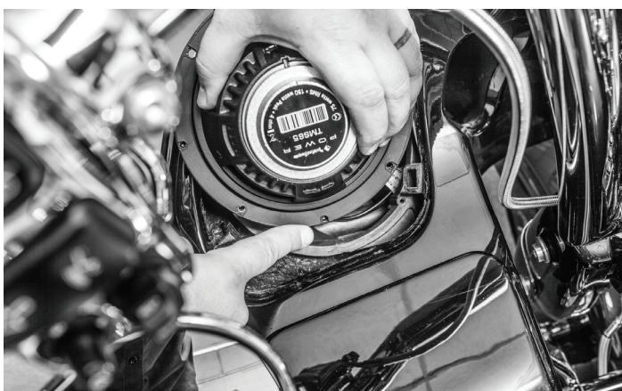
Prior to installing the speaker to the pod, there are alignment pins on the pod that the speaker needs to line up to ensure proper fit.
