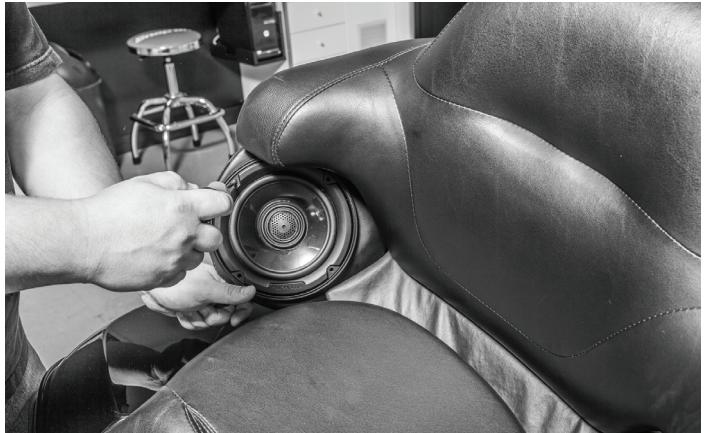
Insert the new Rockford speaker into the speaker pod and secure with mounting screws.
